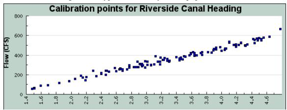
Figure 3 – Typical Calibration Chart
