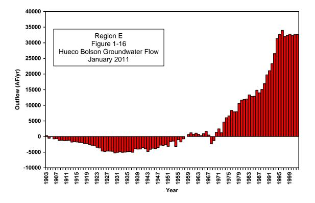
Figure 1-16. Rate of Flow of Hueco Bolson Groundwater from Texas to Mexico
