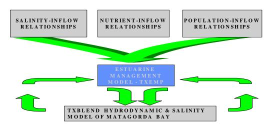
Figure 1.1 Process for Determining Freshwater Inflow Needs.
