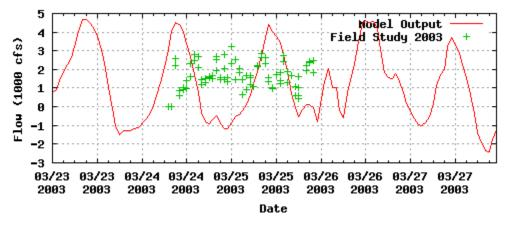
Figure 8.9.i – Measured (green crosses) and Computed (red line) Flows at South Colorado River (Site 7B).
