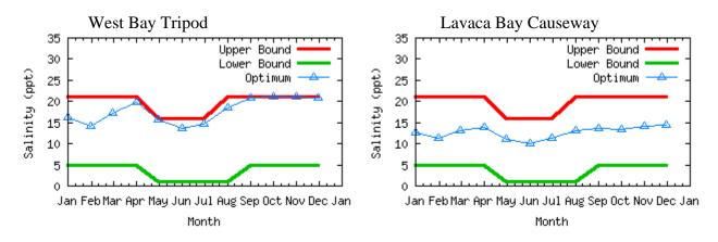
**Figure F.3** Salinity corresponding to optimum flow solutions (Figure F.2) for the constrained optimization problem. Optimum salinity is shown in blue, upper constraint is in red, and lower constraint is in green.
