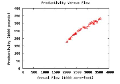
**Figure F.4** Productivity response curve for the loosely constrained optimization problem. Upper flow constraint set to maximum monthly flow. Upper salinity constraint set to 17 ppt from May to July, 22 ppt in remaining months.
