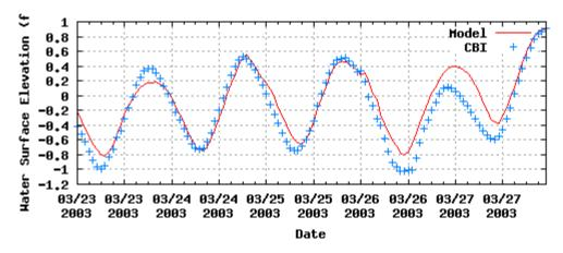
Figure 8.10.b Measured (blue crosses) and Computed (red line) Water Surface Elevation at Port Lavaca (TCOON site 33).
