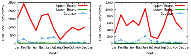
**Figure F.5** Optimum monthly Colorado River (left) and Lavaca River (right) flows for the loosely constrained optimization problem. Optimum solution is shown in blue, upper constraint is in red, and lower constraint is in green.
