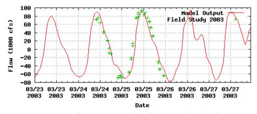
Figure 8.9.b Measured (green crosses) and Computed (red line) Flows at Pass Cavallo (Site 2A).
