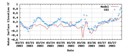
8.10.d Measured (blue crosses) and Computed (red line) Water Surface Elevation at Seadrift (TCOON site 31).
