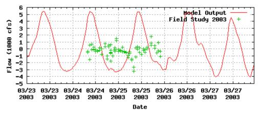
Figure 8.9.1 Measured (green crosses) and Computed (red line) Flows at GIWW West of Bypass Channel (Site 8B).
