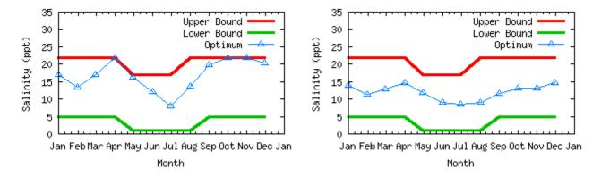
**Figure F.6** Salinity corresponding to optimum flow solutions (Figure F.5) for the loosely constrained optimization problem. Optimum salinity is shown in blue, upper constraint is in red, and lower constraint is in green. West Bay Tripod (left), Lavaca Causeway (right).
