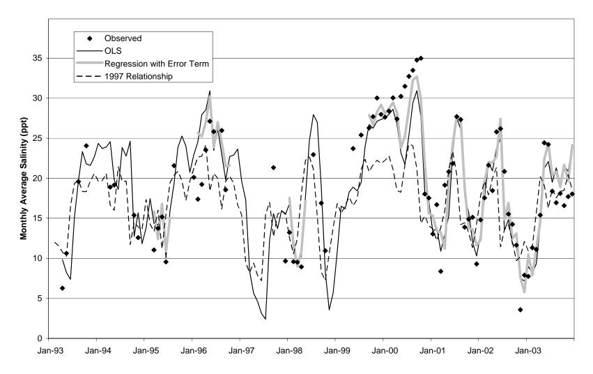
Figure 5.2 Observed and Predicted Salinity for Eastern Matagorda Bay near Mouth of Colorado River (West Bay Tripod) Using Three Models.
