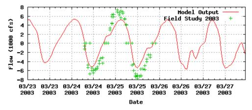
Figure 8.9.m Measured (green crosses) and Computed (red line) Flows at Bypass Channel (Site 8C).
