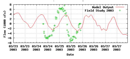
Figure 8.9.k Measured (green crosses) and Computed (red line) Flows at GIWW East of Bypass Channel (Site 8A).
