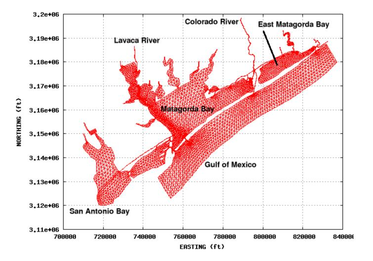
Figure 8.1 TXBLEND Numerical Grid.
