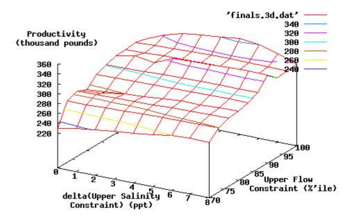
**Figure F.9** Productivity for increased flow and salinity constraints. Salinity constraint change (delta(Upper Salinity Constraint)) represents as increment above 15 ppt for May, June, and July, and 20 ppt for all other months. Flow constraint represents monthly flow percentile. Constrained optimization problem represented by delta(Upper Salinity Constraint) = 0 ppt, Upper Flow Constraint = 70'th percentile
