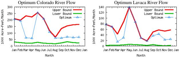
**Figure F.2** Optimum monthly Colorado River and Lavaca River flows for the constrained optimization problem. Optimum solution is shown in blue, upper constraint is in red, and lower constraint is in green.
