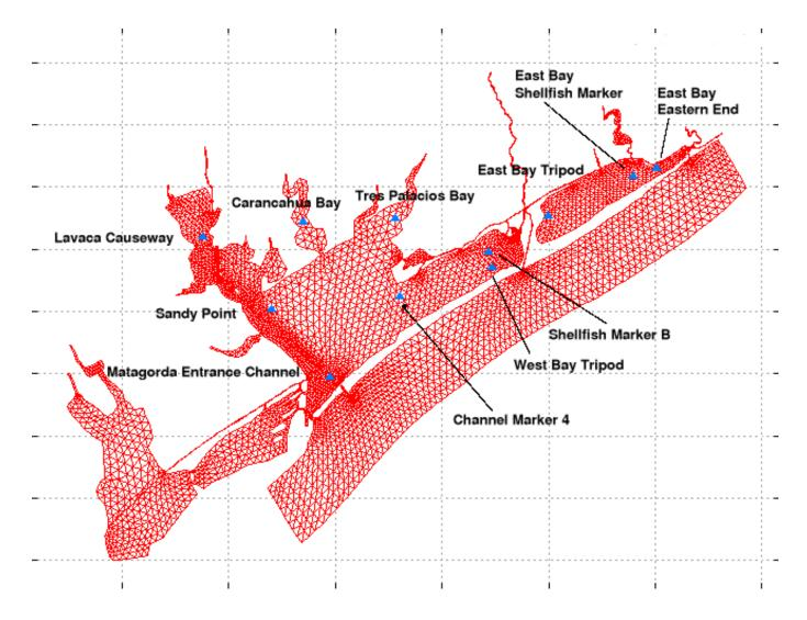
Figure 8.11 Locations of Datasonde Sites (blue triangles) Used in Calibrating TXBLEND.
