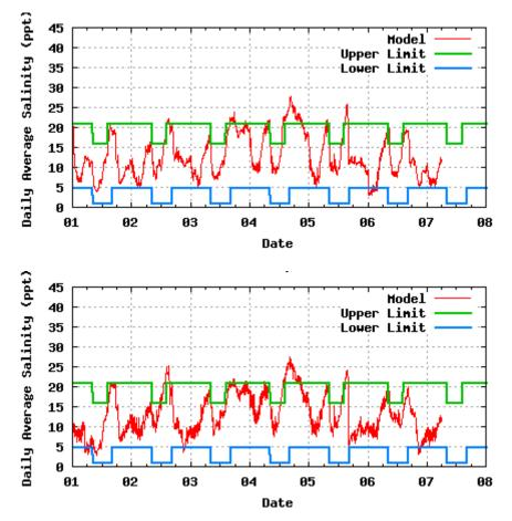
Figure 8.14. Computed Salinity (red) Compared to Target Flow Upper Salinity Constraint (green) and Lower Salinity Constraint (blue) Applied in TXEMP. Model Output for West Bay Tripod (top) and Lavaca Causeway (bottom) Sites.
