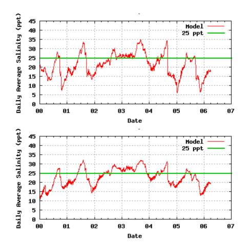
Figure 8.15 Computed Salinity (red) Compared to Critical Flow Salinity Constraint (green) of 25 ppt. Model Output for West Bay Tripod (top) and Lavaca Causeway (bottom) Sites.
