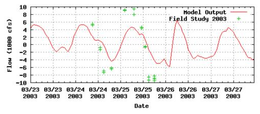
Figure 8.9.d Measured (green crosses) and Computed (red line) Flows at GIWW at Port O'Connor (Site 3B).
