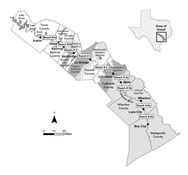
Figure 19-1. Lower Colorado River gain-loss study area, showing outcrops of major and minor aquifers, Colorado River channel, streamflow gauging stations, and study reaches. Source of aquifer outcrop areas: Geologic Atlas Sheets (Bureau of Economic Geology, 1974).
