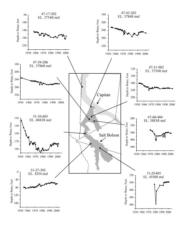
Figure 17-5: Hydrographs from various wells in the Salt Basin area. The Salt Bolson refers the bolson aquifers in the Salt Basin.
