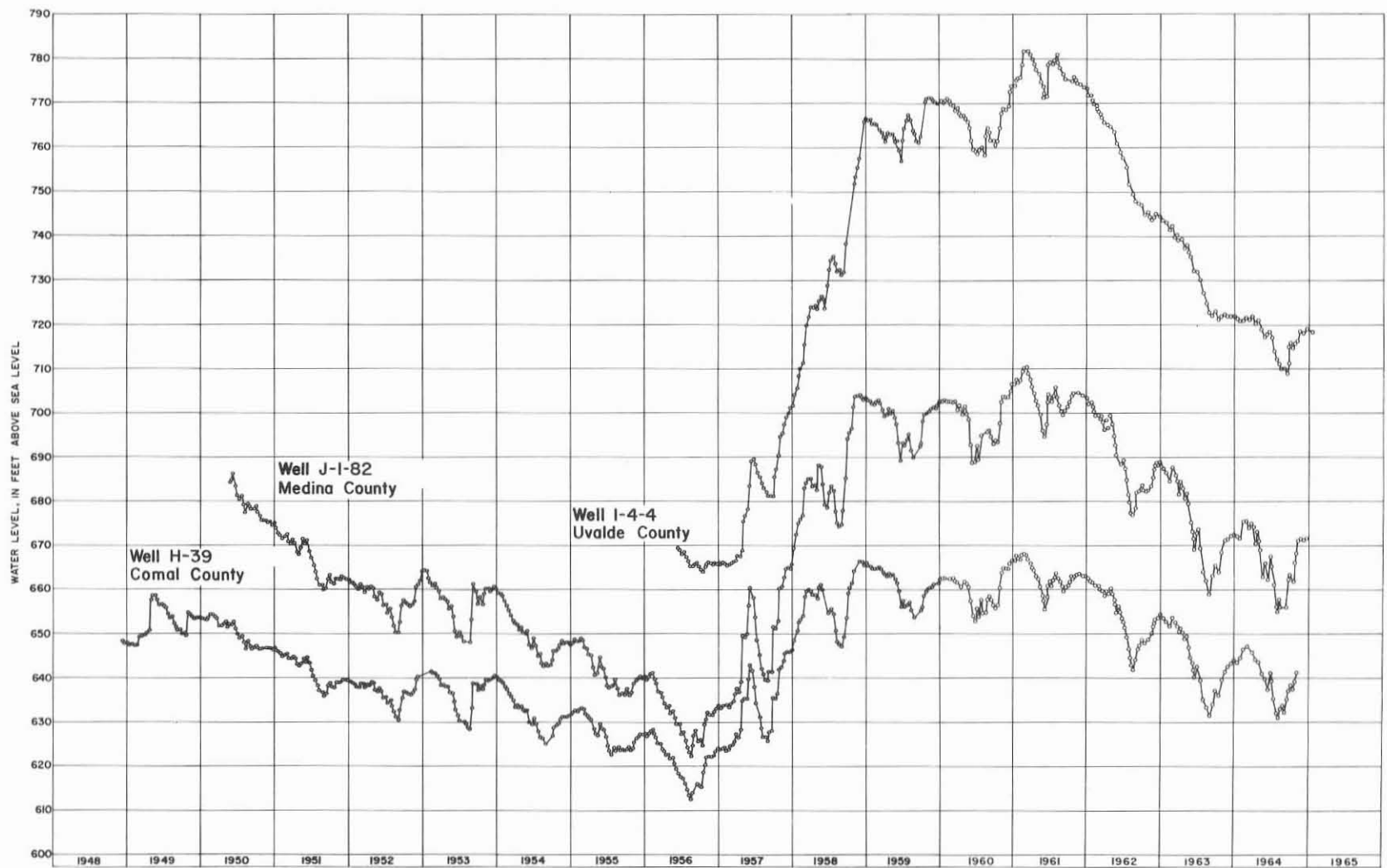
Figure 6 Hydrographs of Representative Wells in the Edwards and Associated Limestones (Sheet 2 of 2)
