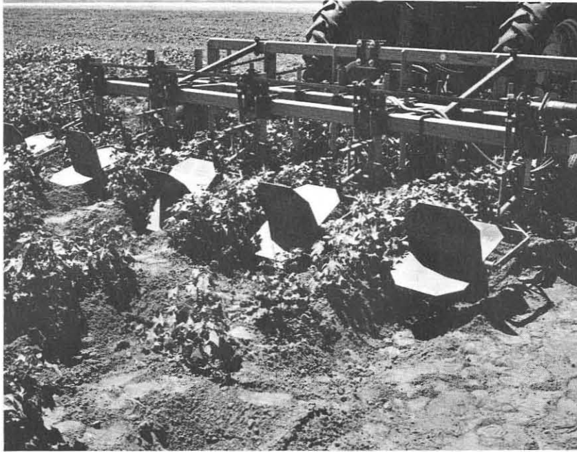
Basin tillage (furrow diker) is used to trap rainfall and hold it for crop use, Hale County.
