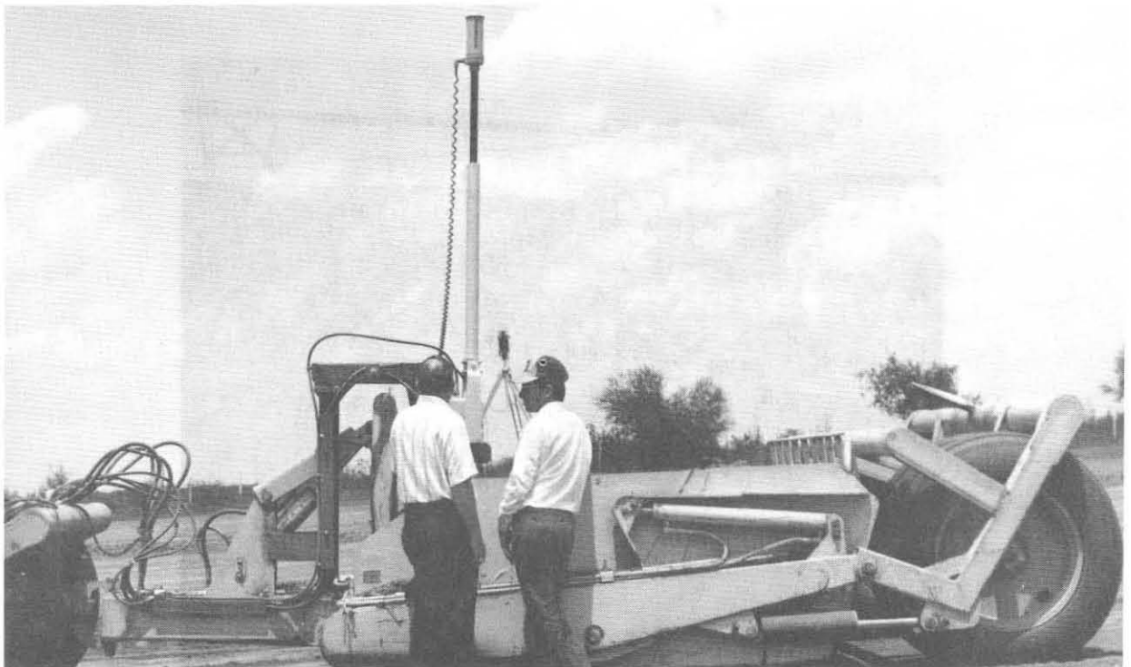
Laser beam "eye" on land leveling equipment, Lower Rio Grande Valley. Photo courtesy U.S. Soil Conservation Service.
