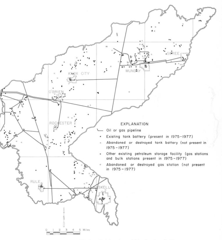
Figure 48. Locations of Pipelines, Tank Batteries, and Other Petroleum Facilities
