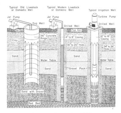
Figure 15. Construction of Wells
