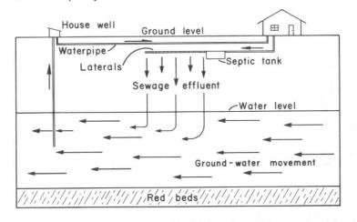
Figure 55. Contamination of a Domestic Ground-Water Supply From a Septic Tank
