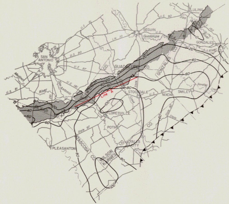
Proposed Line of Wells (Line B) Pumping 20,000 Acre-Feet Per Year Under Artesian Conditions
