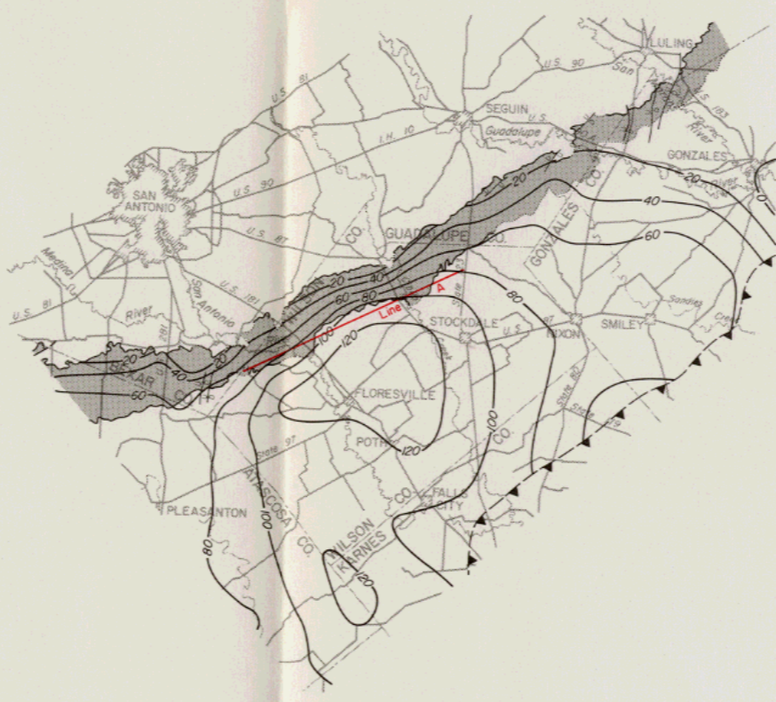
Proposed Line of Wells (Line B) Pumping 30,000 Acre-Feet Per Year Under Artesian Conditions
