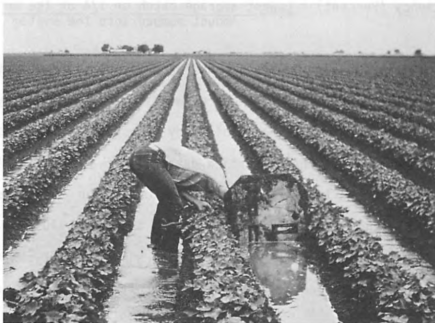
Figure 10 Furrow Evaluation Using an Orifice Plate
