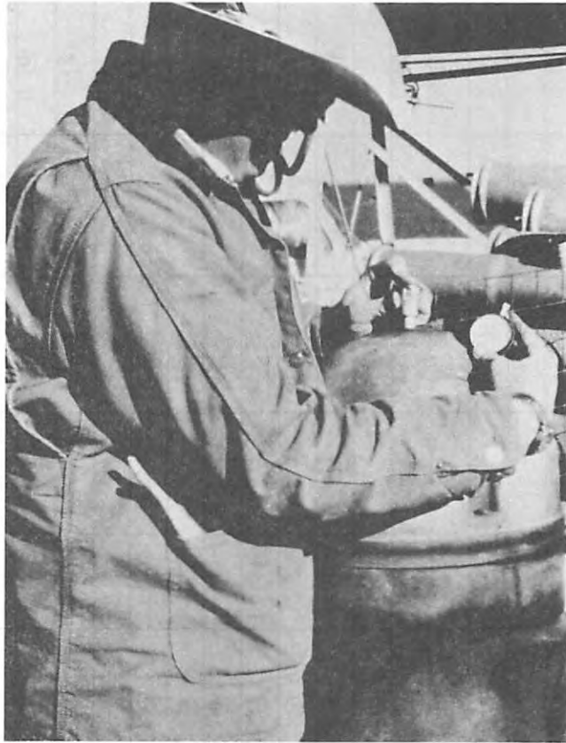
Soil Conservation Service employee checking the gearhead speed (RPM).
