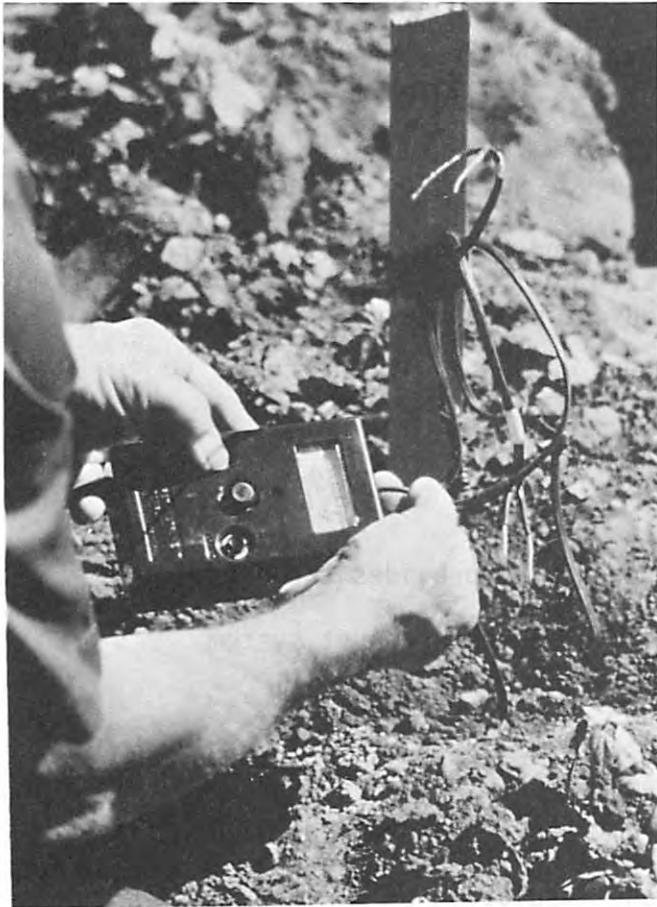
Figure 5 Gypsum Blocks and Meter to Test Soil Moisture
