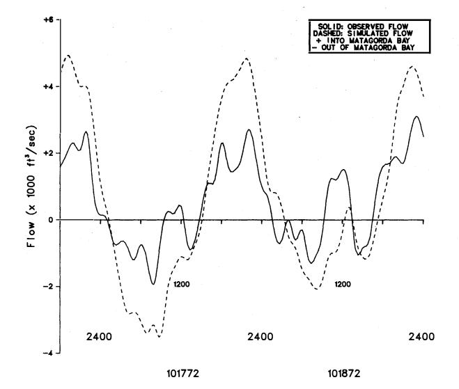
Figure VI. 4. Comparison of Measured and Simulated Flows at Tiger Island Cut.
