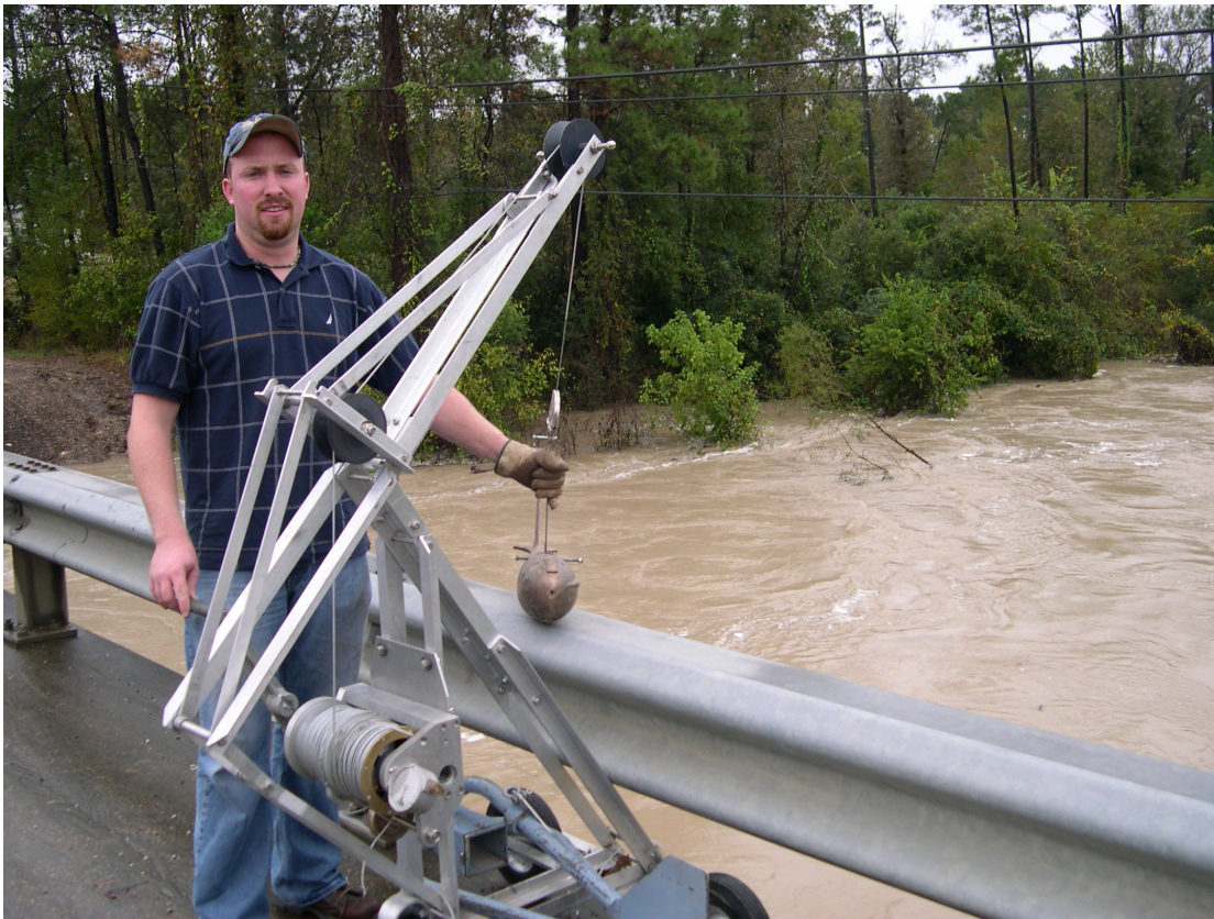
Figure 2. Photograph showing the US D-74 depth-integrating sampler (taken on Long King Creek at Goodrich during the 17-18 November, 2004 storm).
