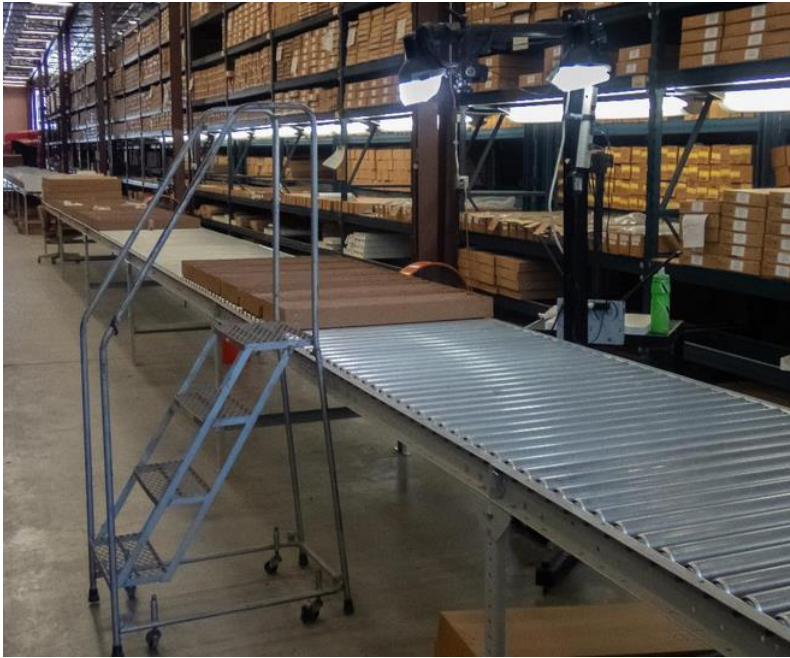
Figure 4-2. CRC warehouse core photography camera mount, with lights and camera mounted.
