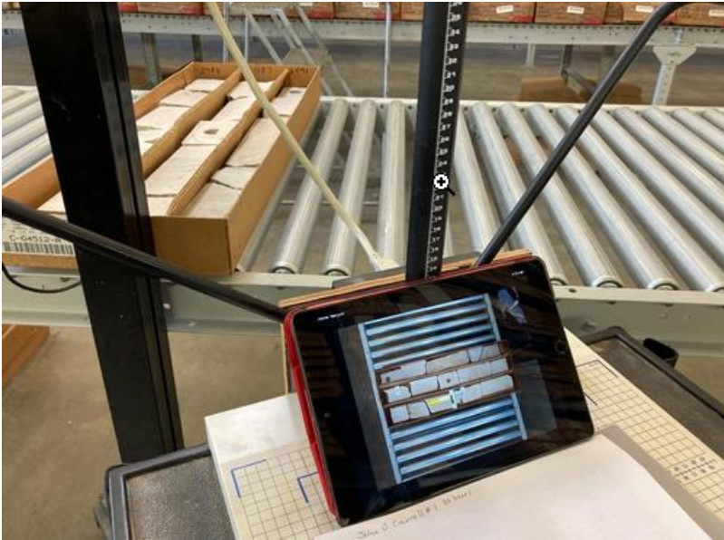
Figure 4-3. Remote view of rock core using Olympus camera Wi-Fi and Olympus O.I. Share software application on Apple iPad. Useful for hands-free viewing of core and orienting slabs to reduce glare.
