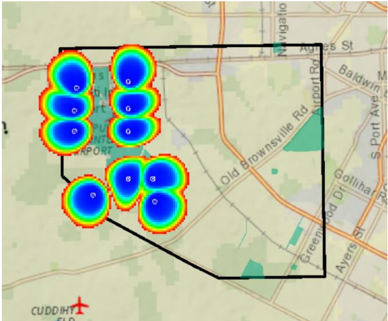
Figure 4-3. Modeled Recharge Extent for Scenario C1-Seasonal Usage after Six Cycles of 2 Year Recharge and 6 Month Recovery (7.9 MGD) Pattern with 10 Phase I wells
