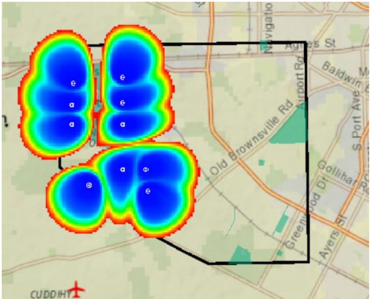
Figure 4-1. Modeled Recharge Extent for Scenario A-Drought Response after Six Cycles of 5 year Recharge and 1.5 Year Recovery Pattern with 10 Phase I wells
