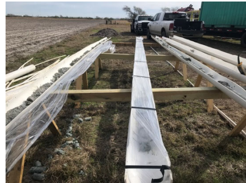
Holders for inspecting and preserving cores during inspection and sampling
