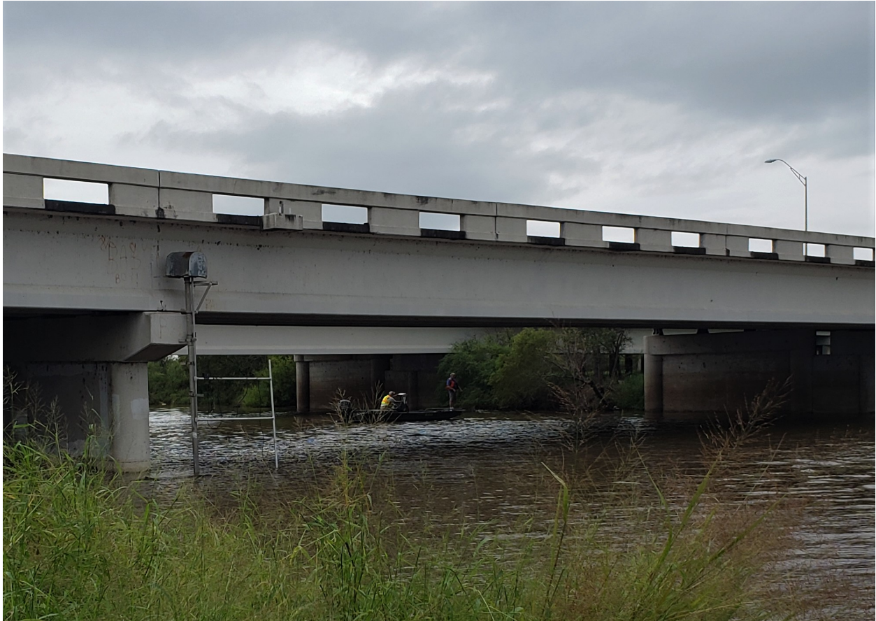
Figure 20. USGS sampling site 08211502 Nueces River at IH37 near Odem, Texas, showing temporary ADVM mount.
