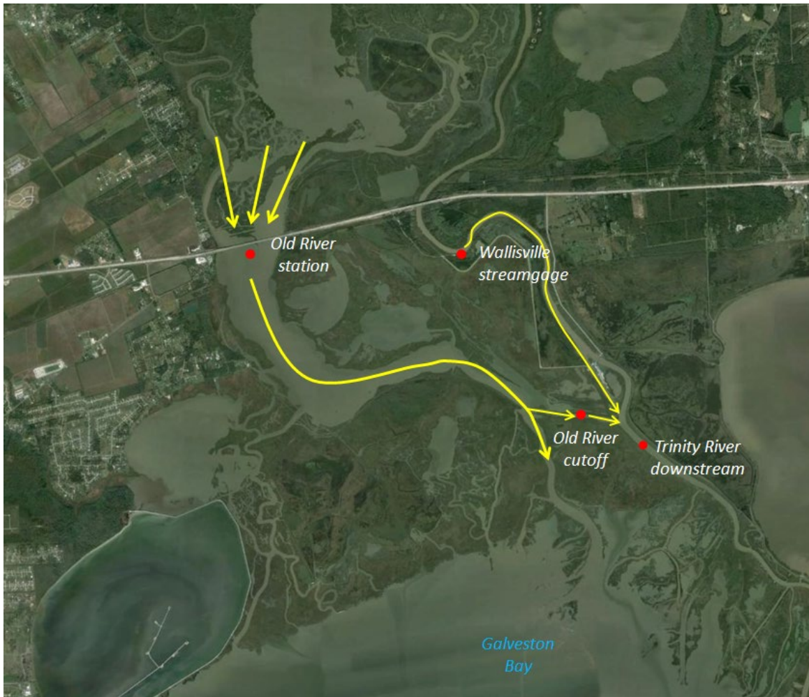
Figure 3. Initial water-quality sampling and discharge measurement locations (red circles) and expected flow patterns (yellow arrows) in the lower Trinity River.
