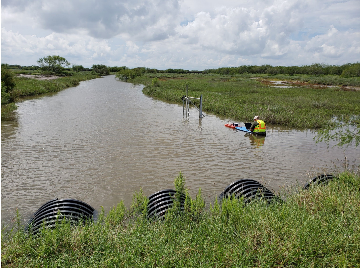
Figure 21. USGS sampling site 0821150305 Rincon Bayou Channel near Odem, Texas, showing semi-permanent ADVm mount.
