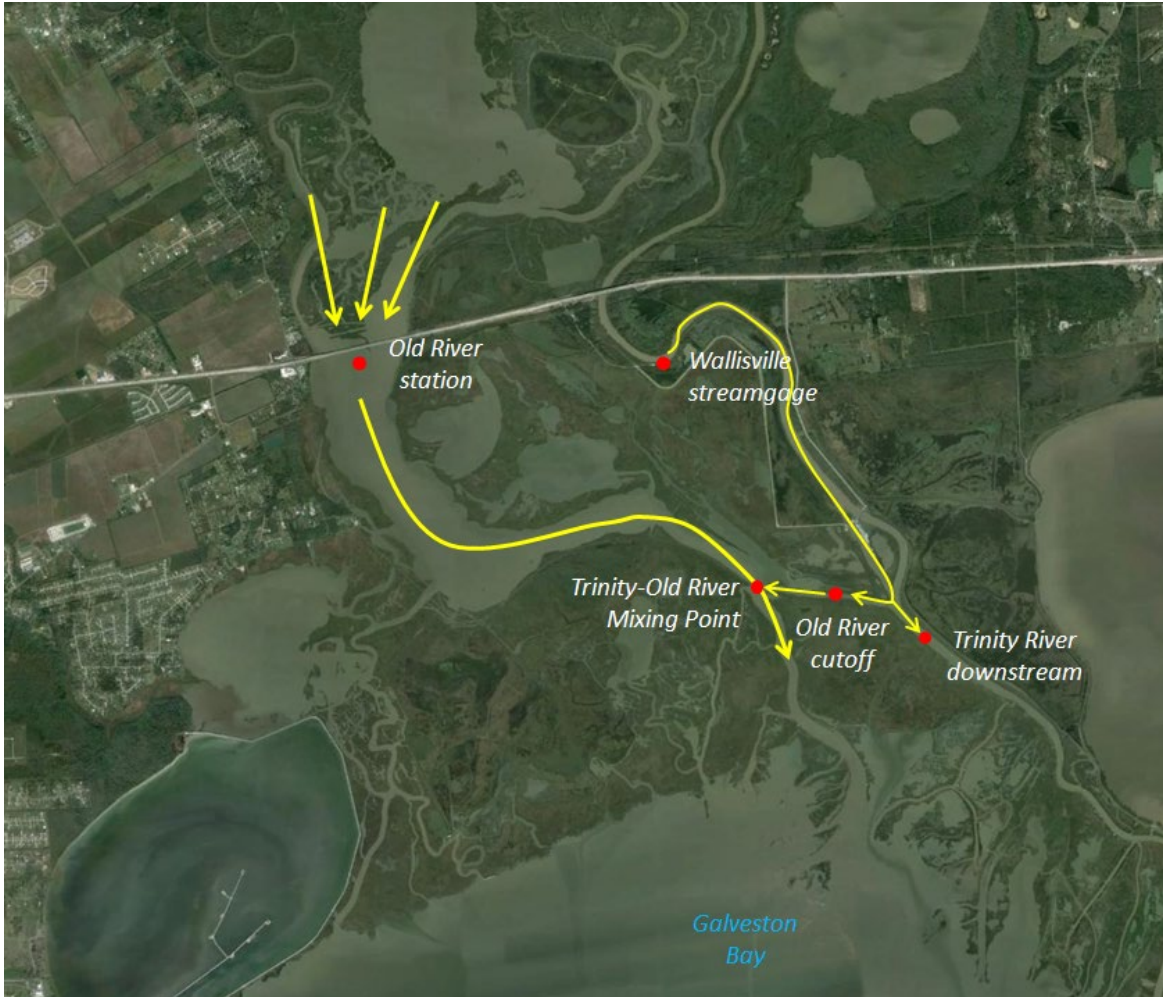
Figure 4. Modified water-quality sampling and discharge measurement locations (red circles) and measured flow patterns (yellow arrows) in the lower Trinity River.
