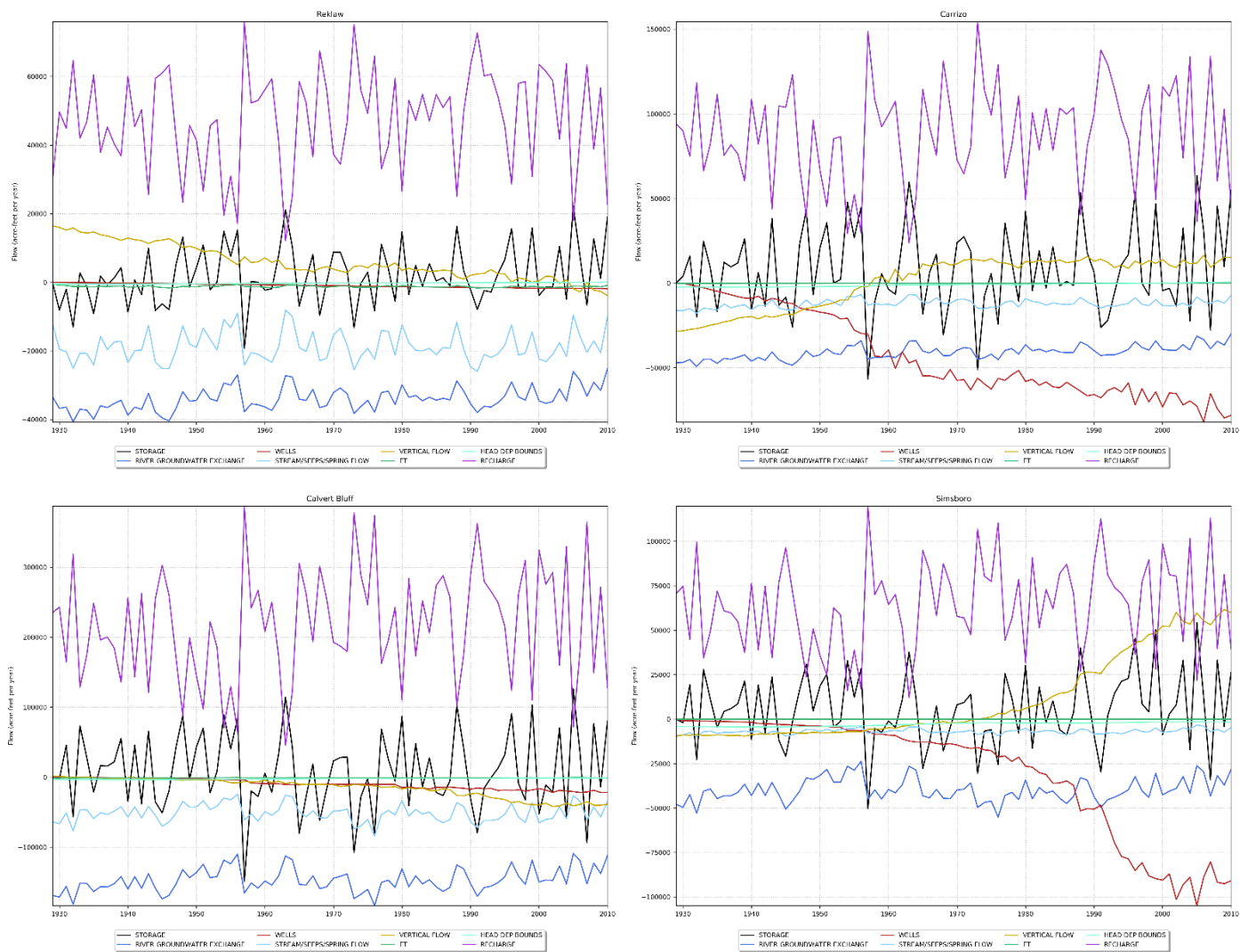
Figure 5.5.2h. Transient water budget for the entire model domain for the Reklaw Formation, Carrizo Aquifer, and Calvert Bluff and Simsboro formations.
