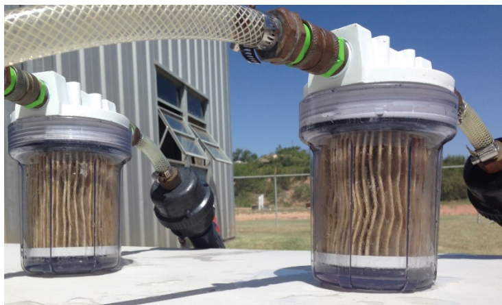
Field-Filtered Virus Sample Collection at Moss Creek Lake Photo Credit: Eva Steinle-Darling
