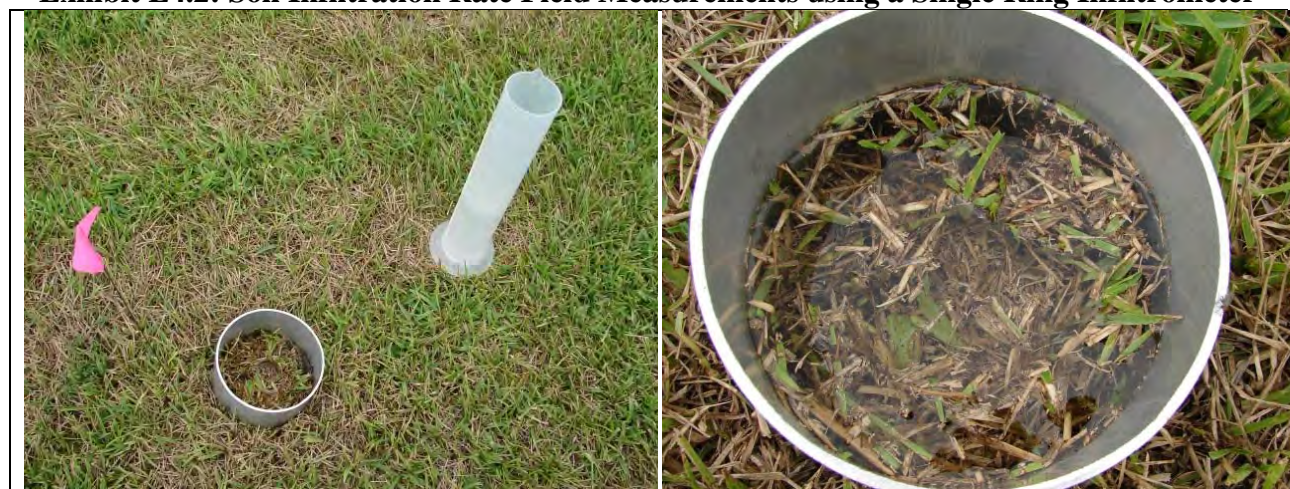
Exhibit L4.2: Soil Infiltration Rate Field Measurements using a Single Ring Infiltrometer
