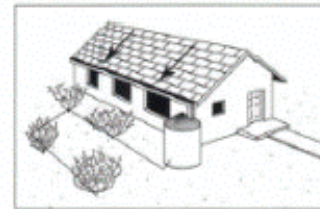
Complex water harvesting system with roof catchment, gutters, downspout, storage and drip distribution system.
