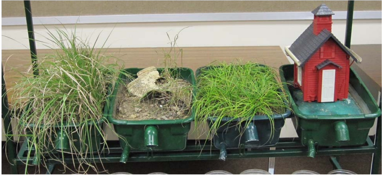
Once the trays and piping have been assembled, they can be filled with “land uses.” In this picture, there are (from left to right) land uses of native grasses, over-grazed land, turf grass, and urban landscape. Note that the water pipes in this example use 45° elbows, which is a viable option.
