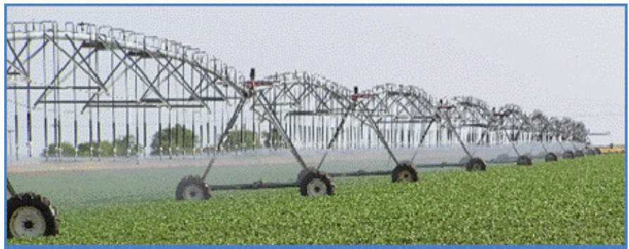
Figure 2.10. Scaled down two-span mini-pivot sprinkler irrigation system. Photo by Justin Mechell.
