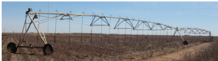
Figure 2.10. Scaled down two-span mini-pivot sprinkler irrigation system. Photo by Justin Mechell.
