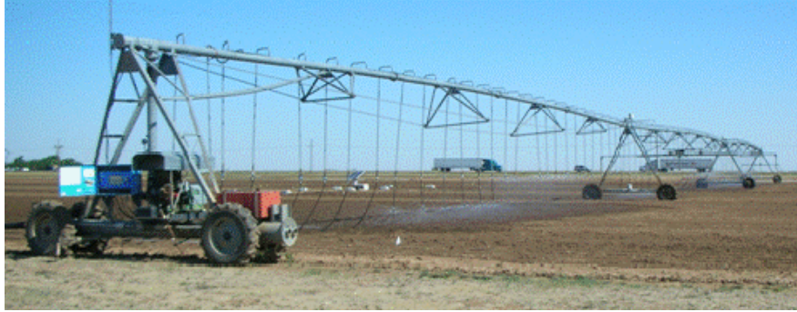
Figure 2.7. Self-propelled linear move sprinkler irrigation system equipped with both LEPA drag hoses and LESA spray nozzles for research conducted at the USDA-ARS Conservation and Production Laboratory at Bushland, TX.
