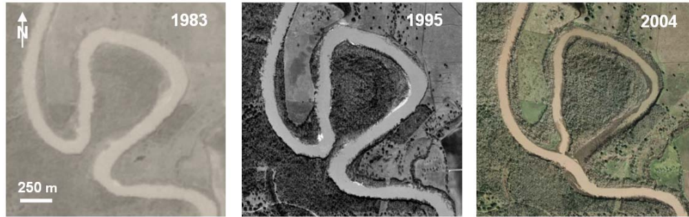
Figure 1.5. The formation of a neck cutoff and an oxbow lake on the Lower Brazos River (LBR), Texas [29°15'38.03"N, 95°34'5.88"W].
