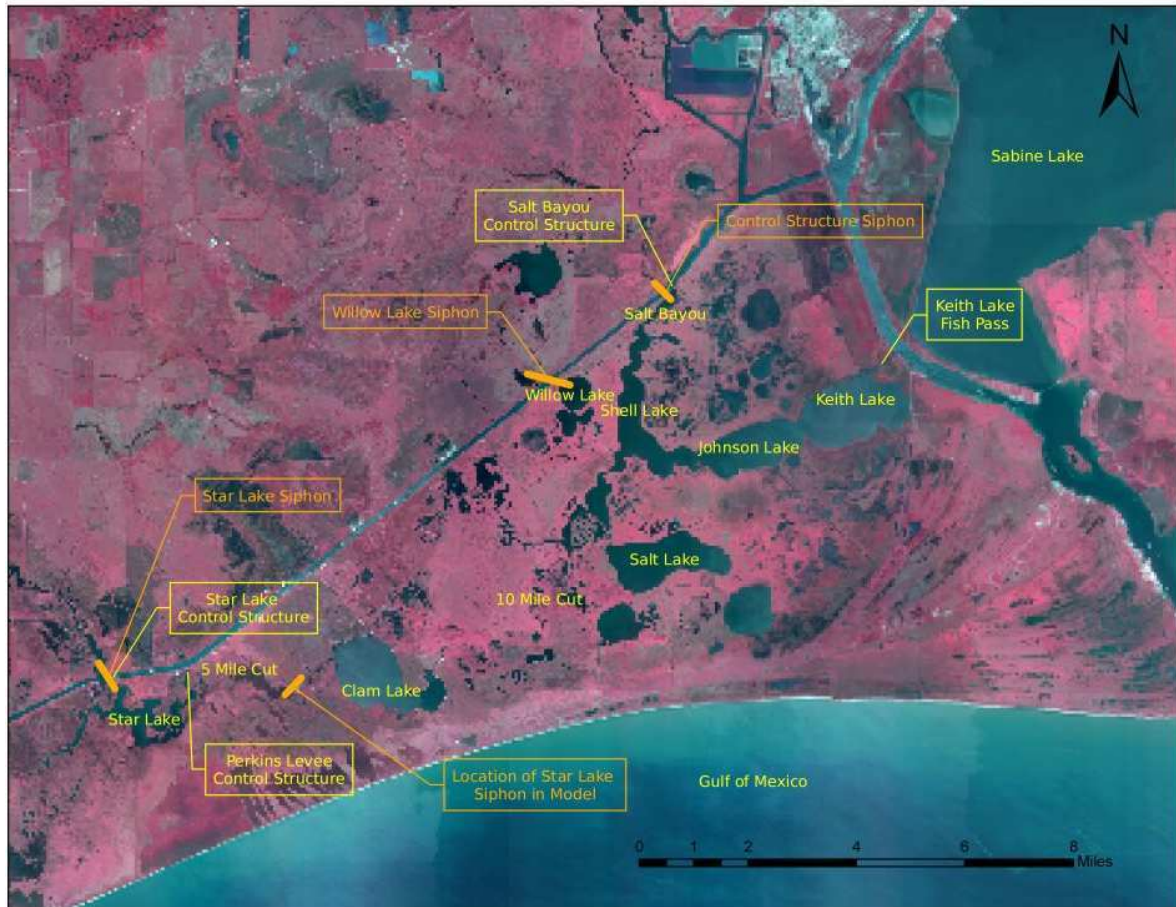
Figure 4.3 Features of the Salt Bayou wetland system along with three proposed freshwater siphon locations, from east to west, Salt Bayou Outfall siphon, Willow Lake Siphon, and the Star Lake siphon. Because Star Lake was not included in the model domain, a fourth location, shown at the lower end of Five-mile Cut, represents the point at which estimated flows from the Star Lake siphon enter the system for model simulation.
