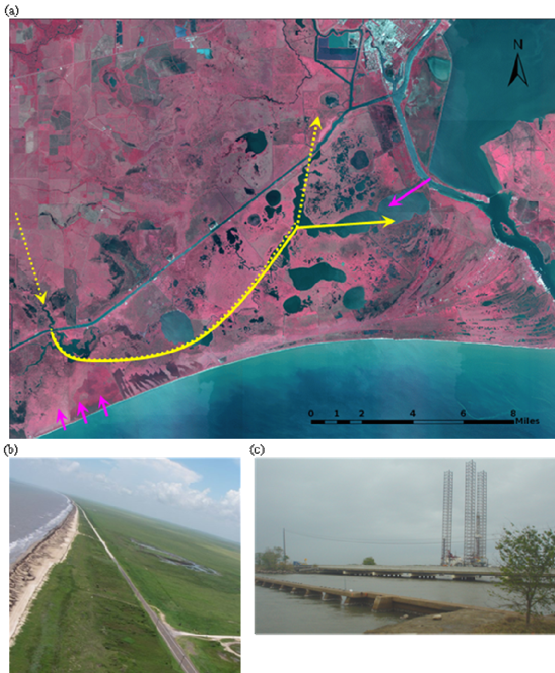
Figure 1.3 a) Historic (dotted yellow) and current (solid yellow) direction of flow in Salt Bayou. Flow of water from the upper watershed was cut off after construction of the GIWW in 1933. Similarly, the natural downstream flow was disrupted. Upon reopening the Fish Pass in 1977, the predominant direction of flow was out through Keith Lake and the Fish Pass. Salinity intrusion to the wetland occurs via the Fish Pass and overtopping events along the beach ridge (pink arrows), b) view of beach ridge west of McFaddin NWR entrance, c) Keith Lake Fish Pass with view of a barge/oil platform passing in the SNWW.
