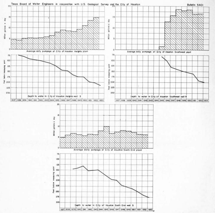
FIGURE 6.— Relation of pumpage to artesian pressure in Houston Heights, Southwest, and South End well fields.
