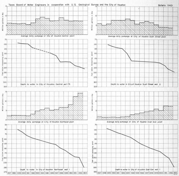
FIGURE 5.- Relation of pumpage to artesian pressure in Houston Central, Scott Street, Northeast, and East End well fields.
