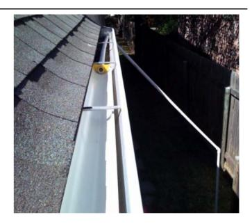
Sampler gutter insert.
