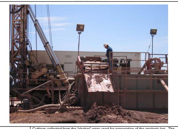
PHOTO NO. 5 DESCRIPTION: Cuttings collected from the "shaker" were used for preparation of the geologic log. The "fines" are separated out by the shaker, thereby biasing the soil samples. Sandy zones (i.e., fines) were noted based on the volume of sand from the sand separator.
