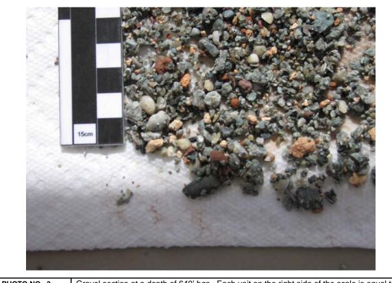
PHOTO NO. 3Gravel section at a depth of 640' bgs. Each unit on the right side of the scale is equal to<br/>1cm.
