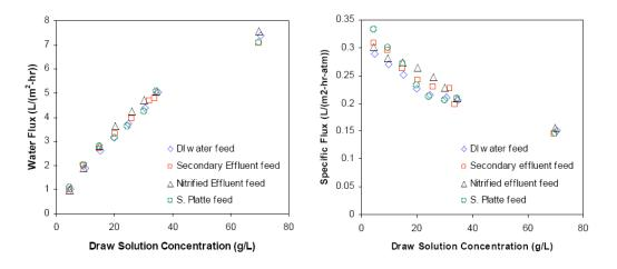
The figure above indicates that at a draw solution concentration of 10 g/L, the expected water flux through the membrane will be 2 L/m<sup>2</sup>-hr, which is equivalent to 1.2 gallon per square foot per day (gfd). Common flux rates for brackish groundwater applications are around 15 gfd (25.5 L/m<sup>2</sup>-hr). At this low flux, membrane area required for a given forward osmosis application is very large, resulting in high capital costs that make this technology economically unfeasible.
