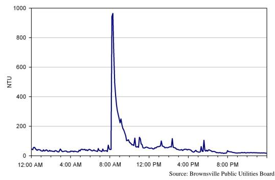
Figure 7 - Snapshot of raw water turbidity spike caused by a passing cargo ship, 12/26/07.
