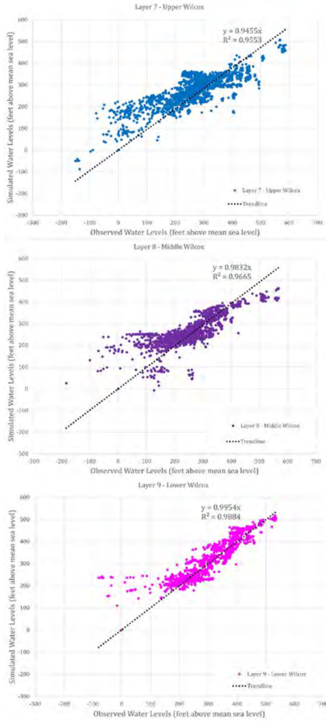
Figure 3.2-15c. Observed vs. Simulated Water Level Elevations for Calibrated 1980 to 2013 Simulation by Layer
