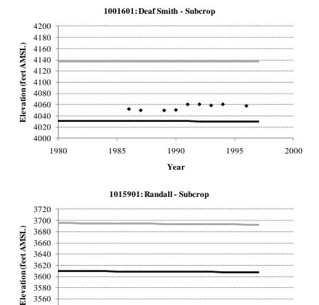
Figure A.1. Simulated and observed water levels for selected wells in the upper portion of the Dockum Aquifer. Dots represent observed values. The black solid line represents simulated water levels in the modified model. The gray solid line represents simulated water levels in the original model (Ewing and others, 2008). All elevations are in feet above mean sea-level.
