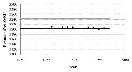
Figure A.2. Simulated and observed water levels for selected wells in the lower portion of the Dockum Aquifer. Dots represent observed values. The black solid line represents simulated water levels in the modified model. The gray solid line represents simulated water levels in the original model (Ewing and others, 2008). All elevations are in feet above mean sea-level.
