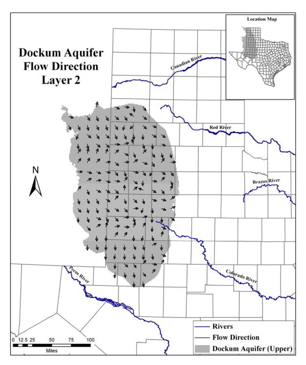
Figure 9. Flow direction for the last year of the model run (1997) for the upper portion of the Dockum Aquifer.
