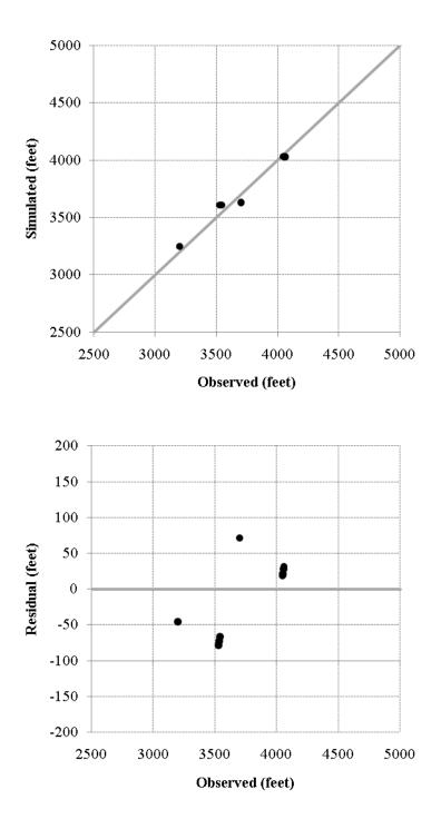
Figure 6. For Layer 2 representing the upper portion of the Dockum Aquifer, plots of (a) simulated versus observed heads, and (b) observed heads versus head residuals.
