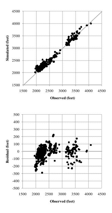
Figure 7. For Layer 3 representing the lower portion of the Dockum Aquifer, plots of (a) simulated versus observed heads, and (b) observed heads versus head residuals.
