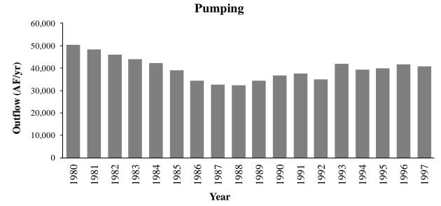
Figure 12. Pumping through time for the historical portion of the modified groundwater model of the Dockum Aquifer. Flow volumes are in acre-feet per year and represent the entire model.
