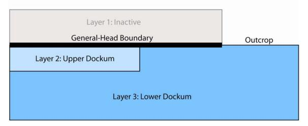
Figure 5. Difference in design of the groundwater models for the Dockum aquifer between the original model (Ewing and others, 2008) and the modified model.
