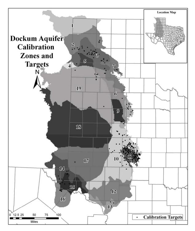
Figure 4. Calibration zones and targets used in the modified Dockum Aquifer groundwater model
