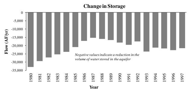
Figure 13. Change in the volume of water stored in the Dockum Aquifer through time for the historical portion of the modified groundwater model. Flow volumes are in acre-feet per year and represent the entire model.
