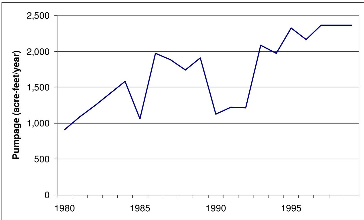
Figure A-4- Pumpage in Brown County included in the groundwater availability model for the northern part of the Trinity Aquifer.
