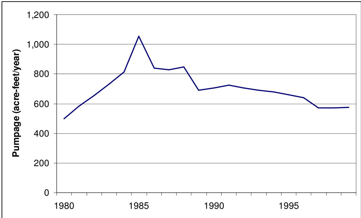
Figure A-5- Pumpage in Burnet County included in the groundwater availability model for the northern part of the Trinity Aquifer.
