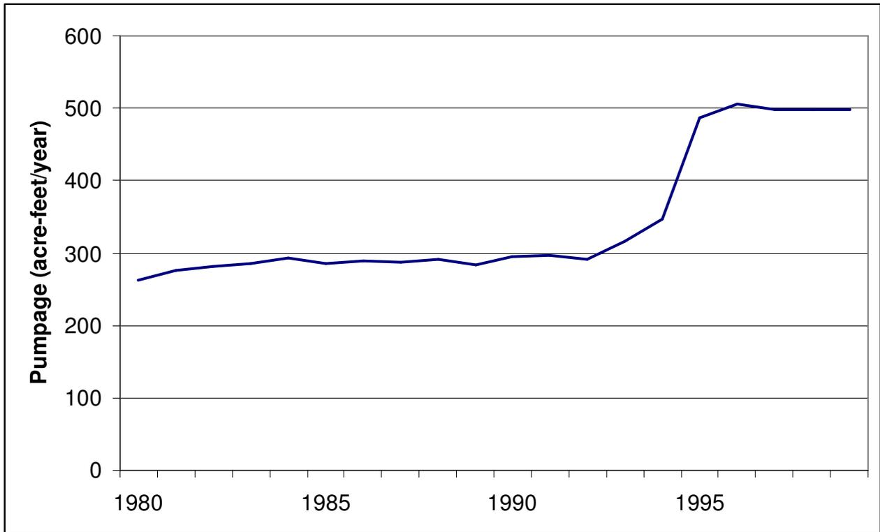
Figure A-33- Pumpage in Montague County included in the groundwater availability model for the northern part of the Trinity Aquifer.
