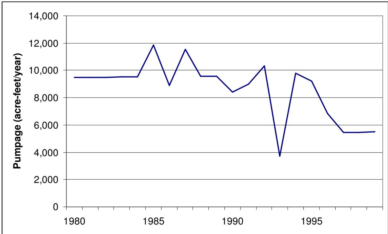
Figure A-13- Pumpage in Eastland County included in the groundwater availability model for the northern part of the Trinity Aquifer.
