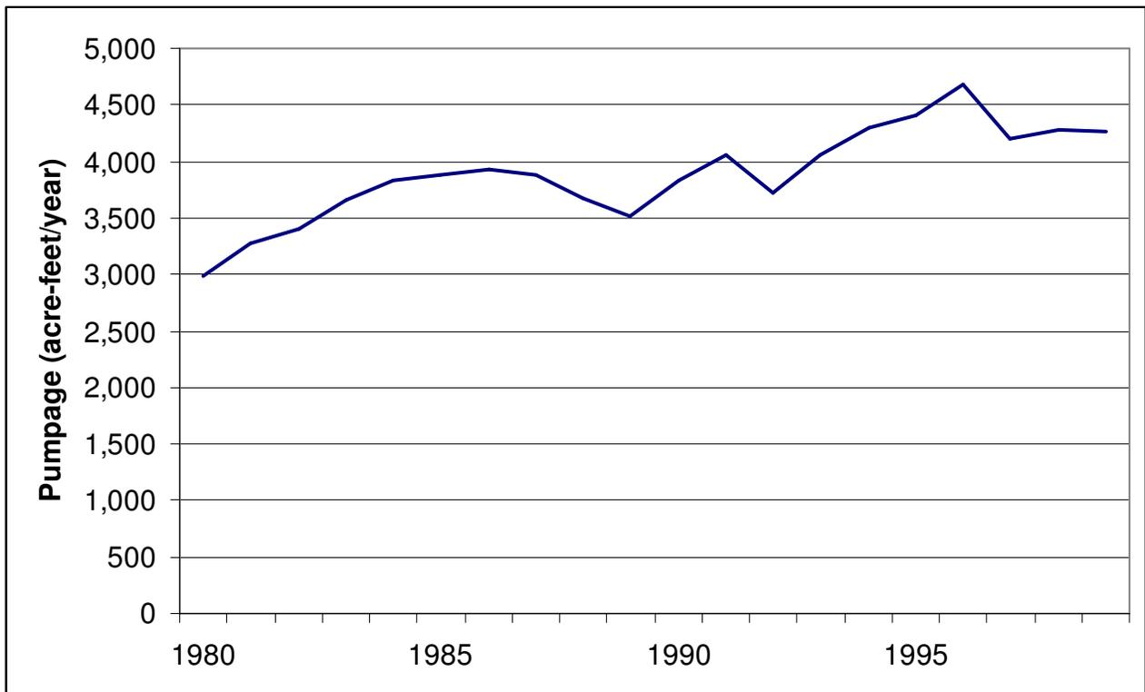
Figure A-44- Pumpage in Wise County included in the groundwater availability model for the northern part of the Trinity Aquifer.
