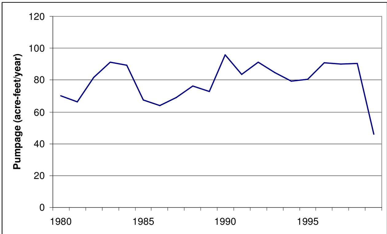
Figure A-34- Pumpage in Navarro County included in the groundwater availability model for the northern part of the Trinity Aquifer.
