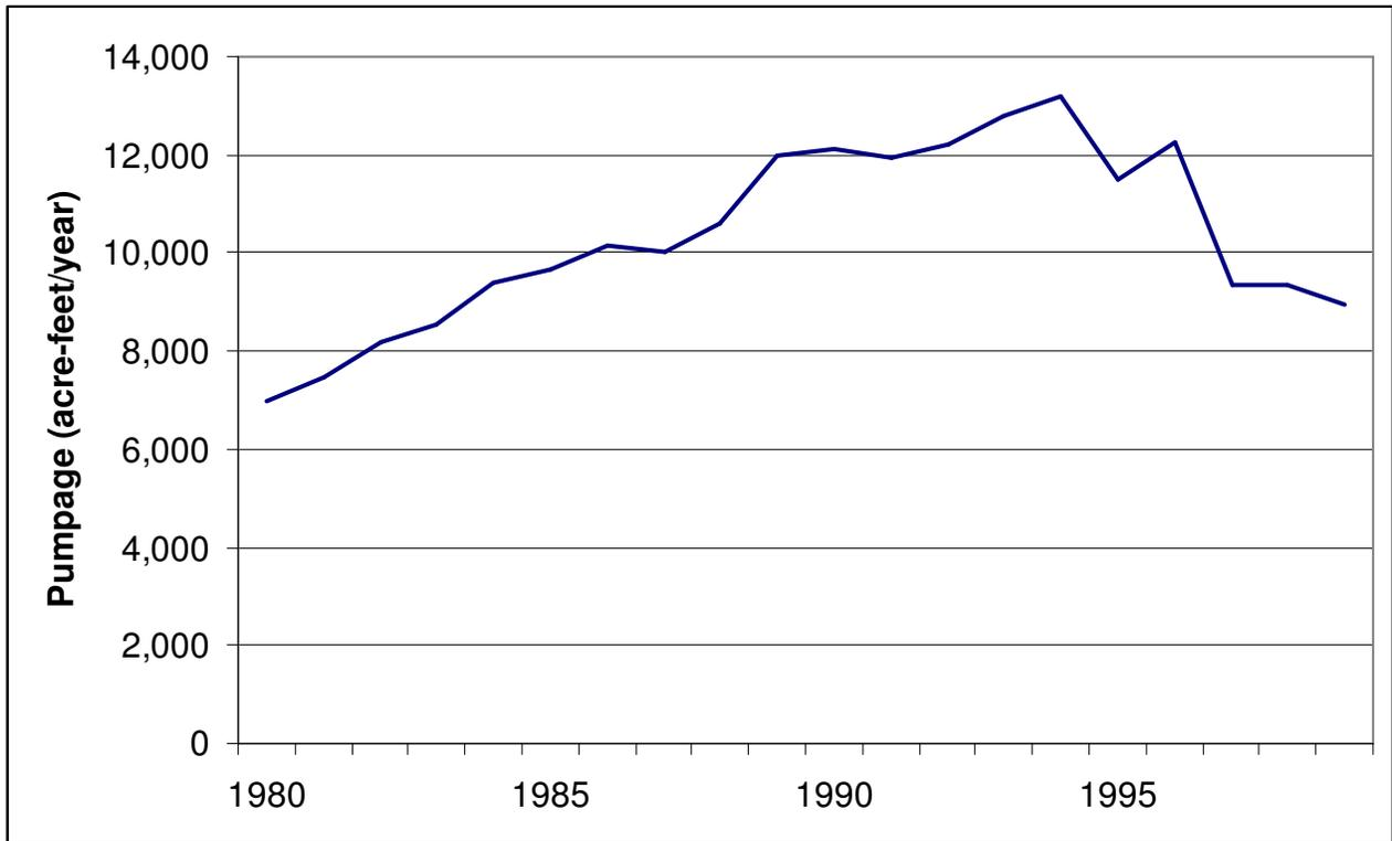
Figure A-43- Pumpage in Williamson County included in the groundwater availability model for the northern part of the Trinity Aquifer.
