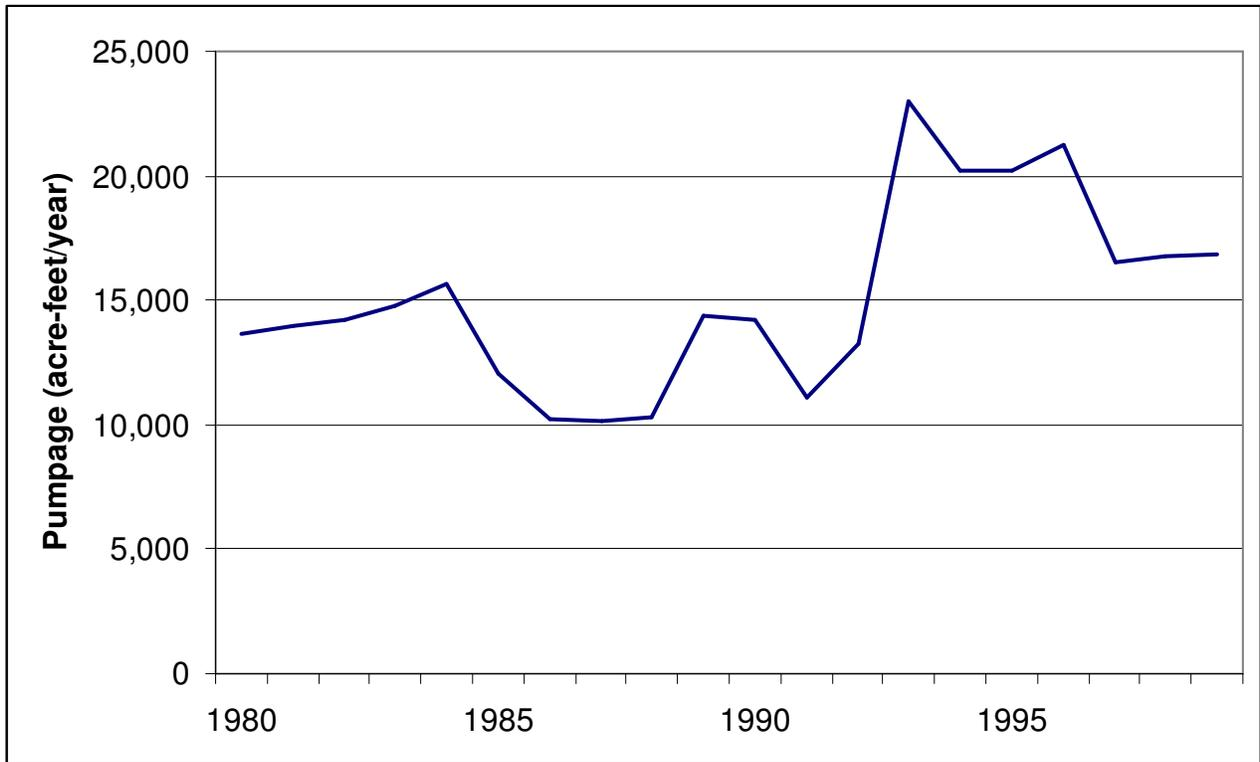
Figure A-15- Pumpage in Erath County included in the groundwater availability model for the northern part of the Trinity Aquifer.
