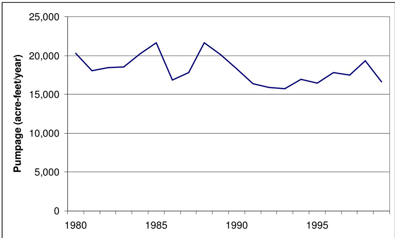
Figure A-40- Pumpage in Tarrant County included in the groundwater availability model for the northern part of the Trinity Aquifer.
