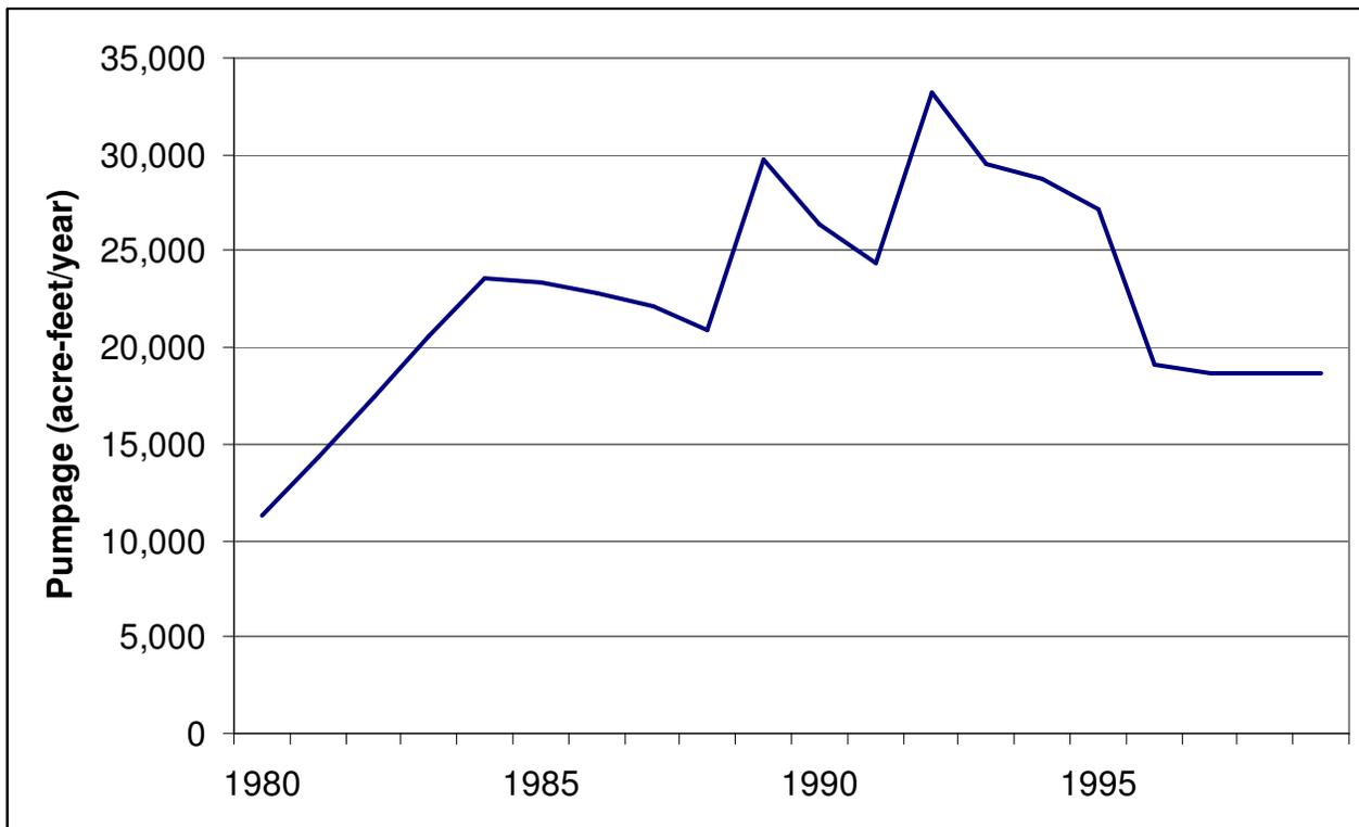
Figure A-8- Pumpage in Comanche County included in the groundwater availability model for the northern part of the Trinity Aquifer.
