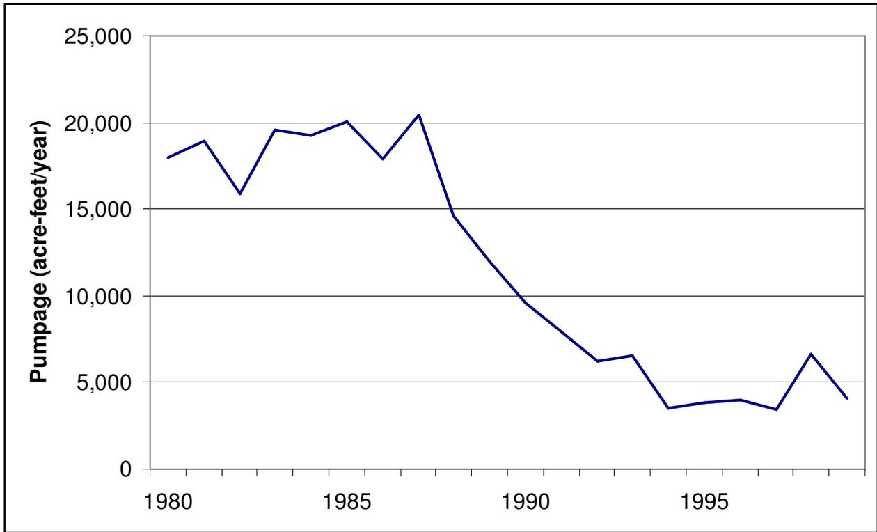
Figure A-11- Pumpage in Dallas County included in the groundwater availability model for the northern part of the Trinity Aquifer.
