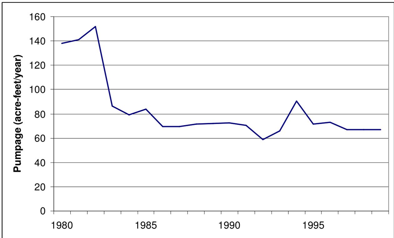
Figure A-16- Pumpage in Falls County included in the groundwater availability model for the northern part of the Trinity Aquifer.
