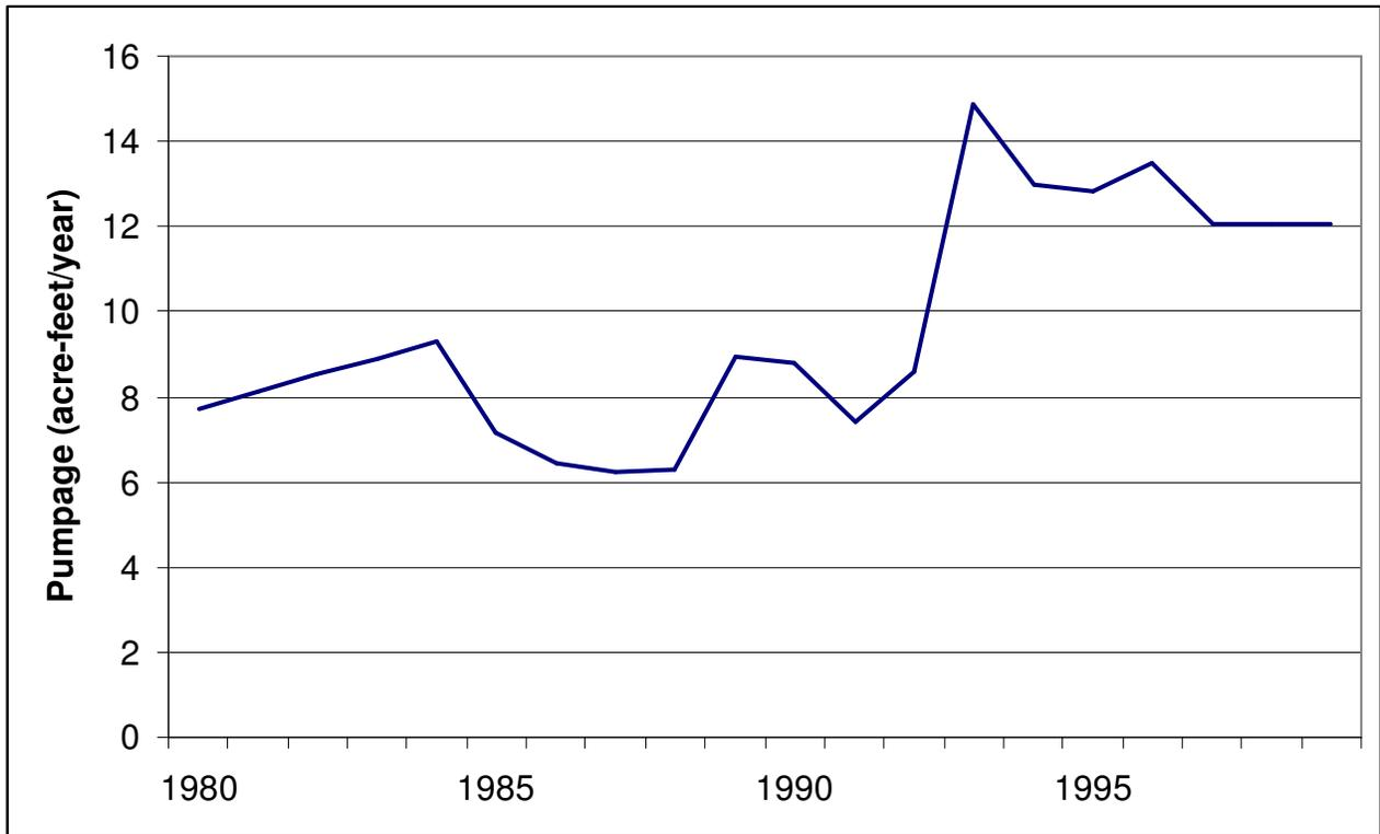
Figure A-35- Pumpage in Palo Pinto County included in the groundwater availability model for the northern part of the Trinity Aquifer.
