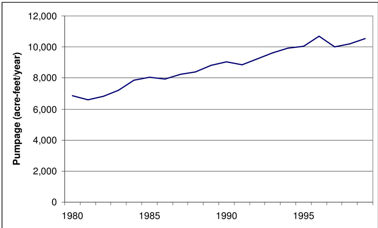
Figure A-24- Pumpage in Johnson County included in the groundwater availability model for the northern part of the Trinity Aquifer.
