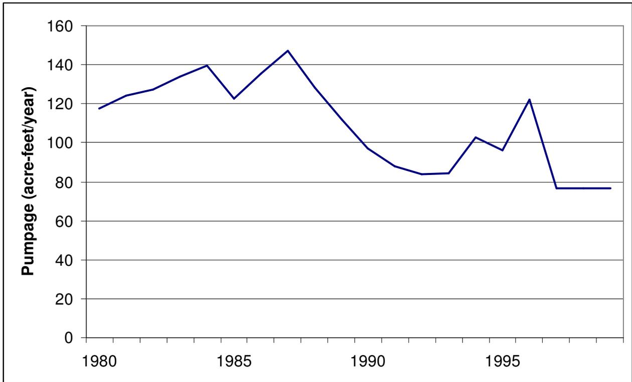
Figure A-25- Pumpage in Kaufman County included in the groundwater availability model for the northern part of the Trinity Aquifer.
