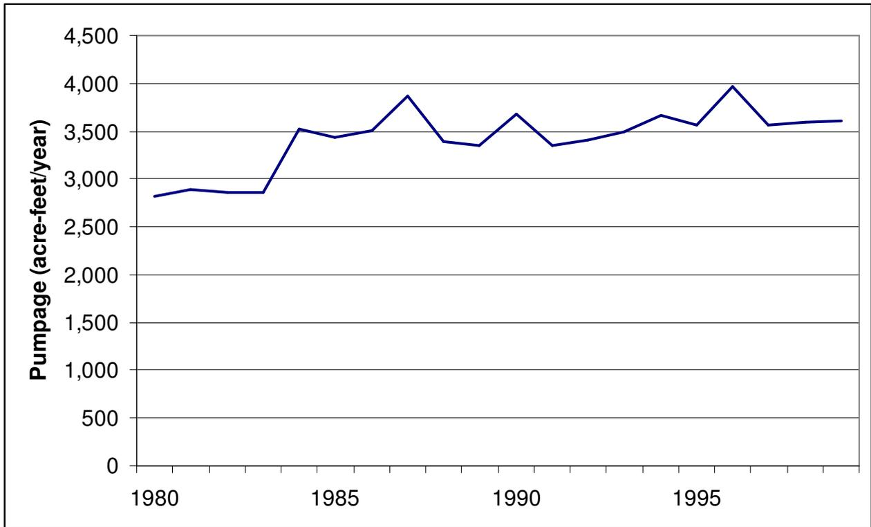
Figure A-3- Pumpage in Bosque County included in the groundwater availability model for the northern part of the Trinity Aquifer.
