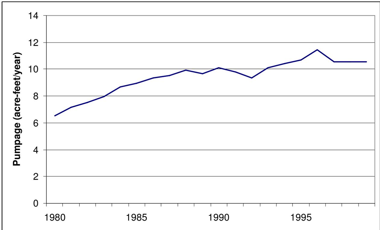
Figure A-23- Pumpage in Jack County included in the groundwater availability model for the northern part of the Trinity Aquifer.
