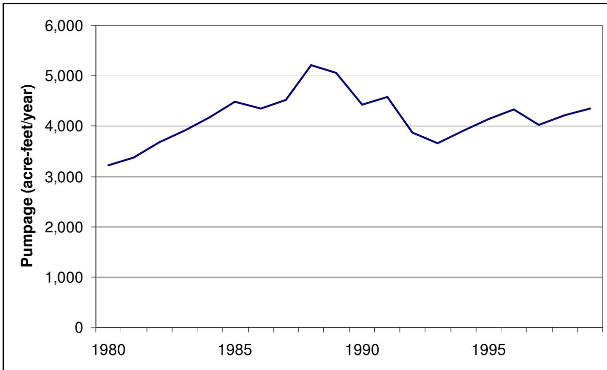
Figure A-7- Pumpage in Collin County included in the groundwater availability model for the northern part of the Trinity Aquifer.
