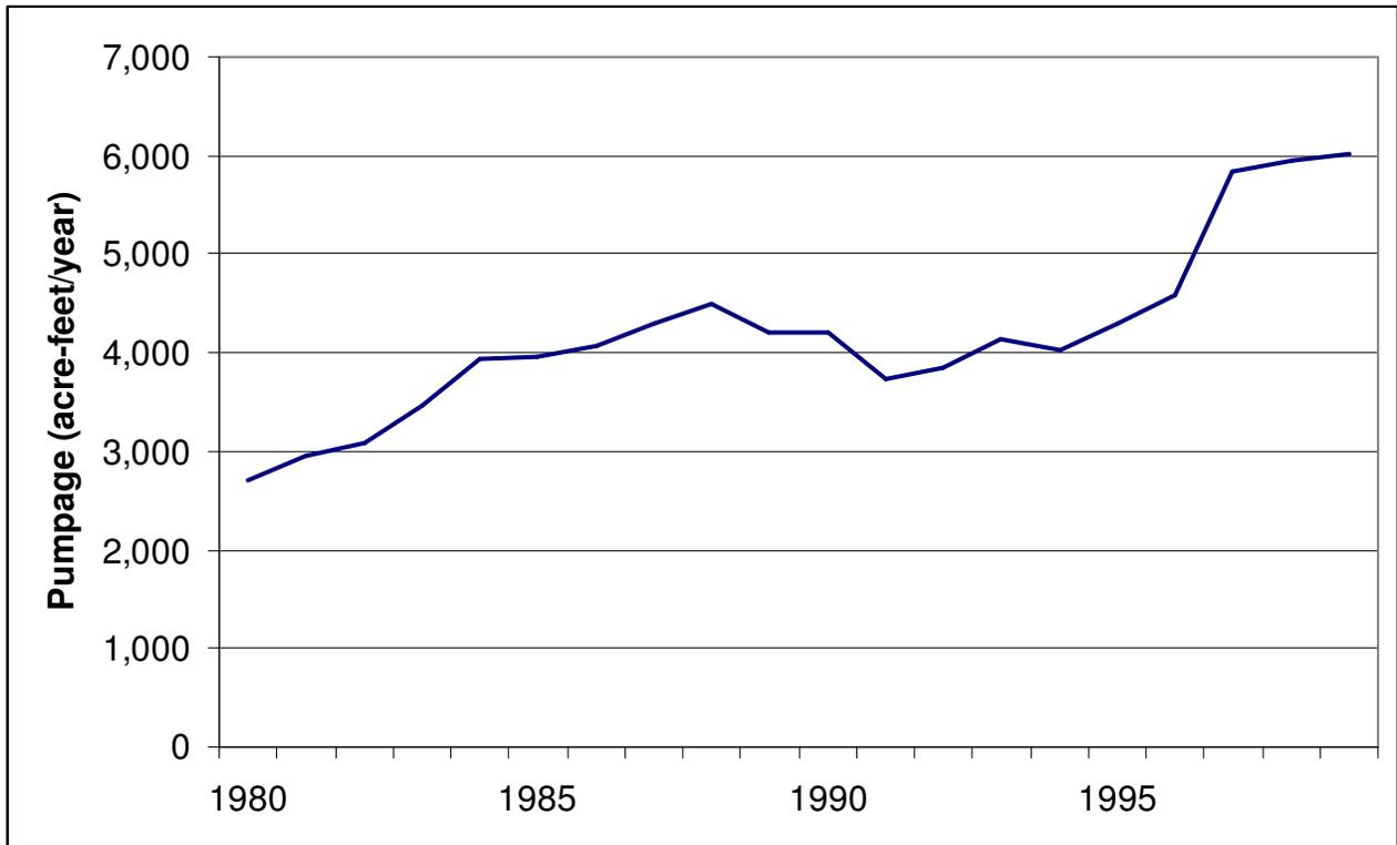
Figure A-21- Pumpage in Hood County included in the groundwater availability model for the northern part of the Trinity Aquifer.
