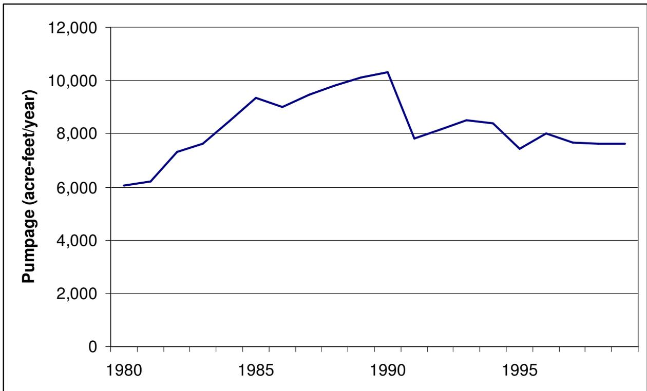
Figure A-14- Pumpage in Ellis County included in the groundwater availability model for the northern part of the Trinity Aquifer.
