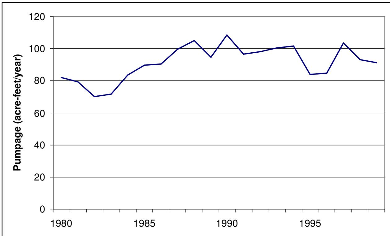
Figure A-22- Pumpage in Hunt County included in the groundwater availability model for the northern part of the Trinity Aquifer.
