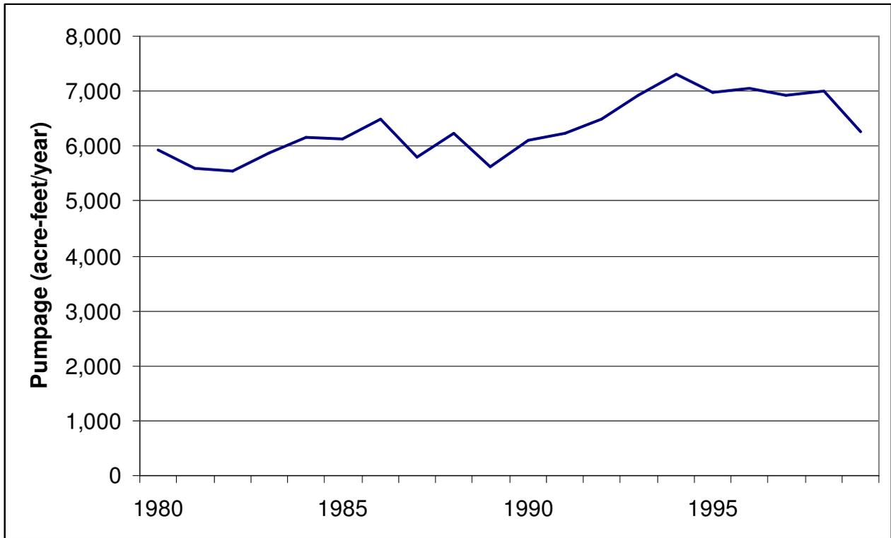
Figure A-9- Pumpage in Cooke County included in the groundwater availability model for the northern part of the Trinity Aquifer.
