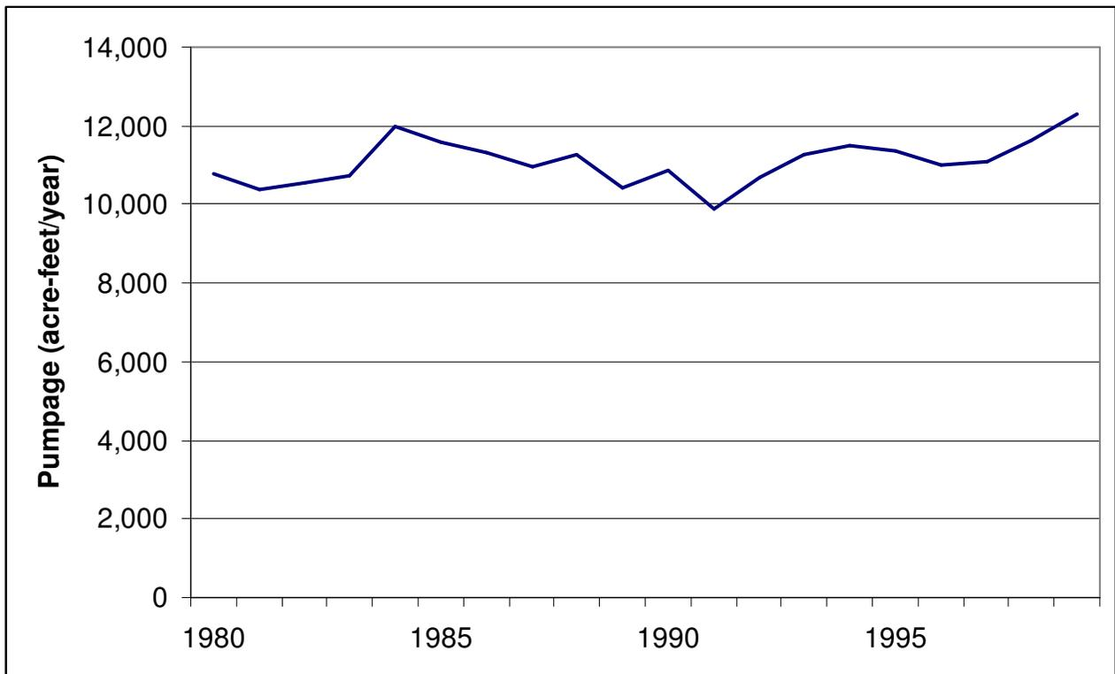
Figure A-30- Pumpage in McLennan County included in the groundwater availability model for the northern part of the Trinity Aquifer.
