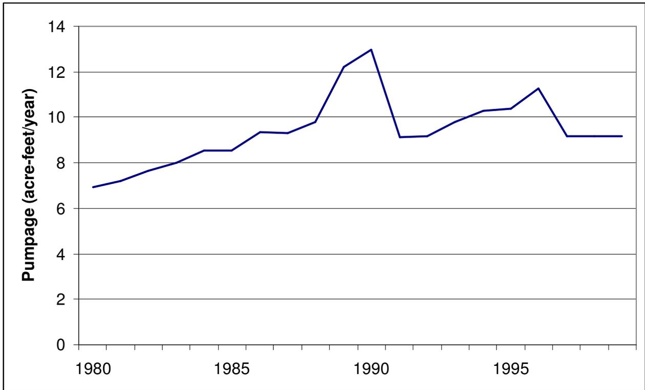
Figure A-31- Pumpage in Milam County included in the groundwater availability model for the northern part of the Trinity Aquifer.
