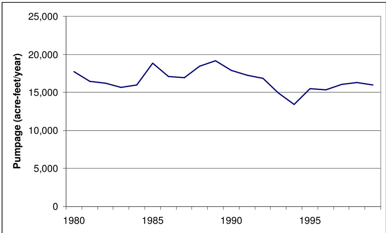
Figure A-18- Pumpage in Grayson County included in the groundwater availability model for the northern part of the Trinity Aquifer.
