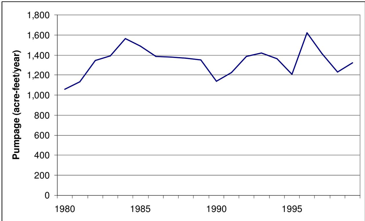
Figure A-39- Pumpage in Somervell County included in the groundwater availability model for the northern part of the Trinity Aquifer.
