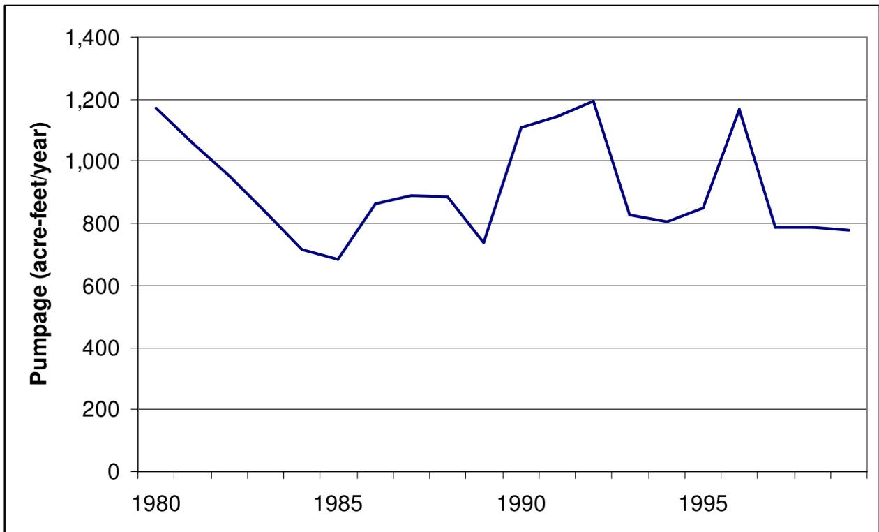
Figure A-32- Pumpage in Mills County included in the groundwater availability model for the northern part of the Trinity Aquifer.
