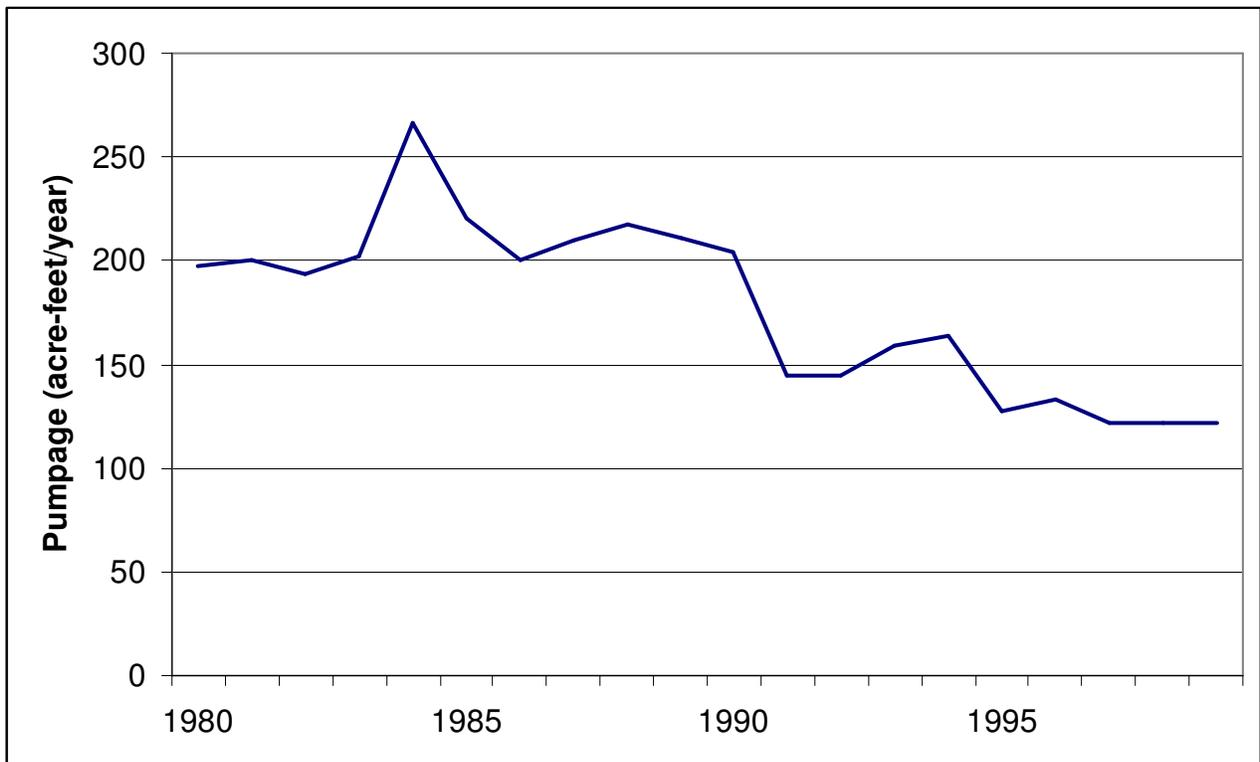
Figure A-26- Pumpage in Lamar County included in the groundwater availability model for the northern part of the Trinity Aquifer.
