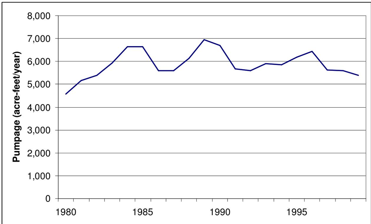
Figure A-42- Pumpage in Travis County included in the groundwater availability model for the northern part of the Trinity Aquifer.
