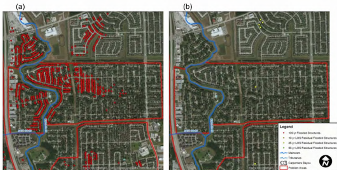
Figure 23: Target LOS alternative Analysis for PA03 (a) 100-year computed flooded structures (b) Computed residual flooded structures after 25-year LOS for PA03
