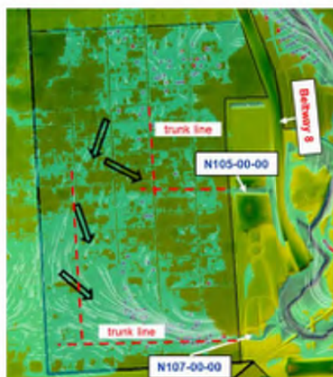
Figure 34: Suggested drainage improvement to PA04: Centered trunk lines to capture lateral flow
