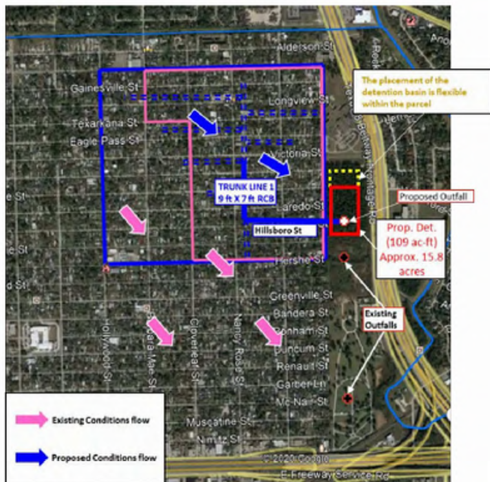
Figure 3. Existing and Proposed Conditions drainage boundaries
