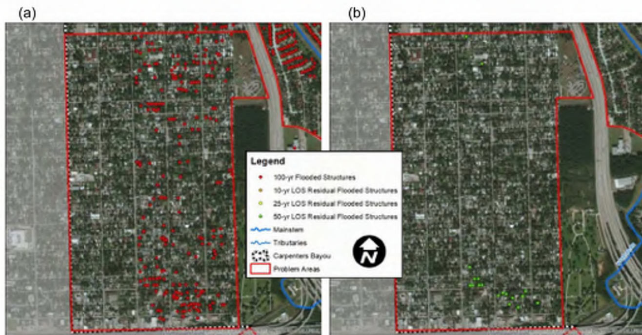
Figure 31: Target LOS alternative Analysis for PA04 (a) 100-year computed flooded structures (b) Computed residual flooded structures after 50-year LOS for PA04
