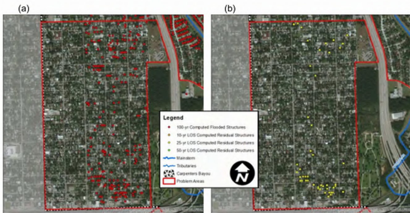
Figure 29: Reduced LOS alternative Analysis for PA04 (a) 100-year computed flooded structures (b) Computed residual flooded structures after 25-year LOS for PA04
