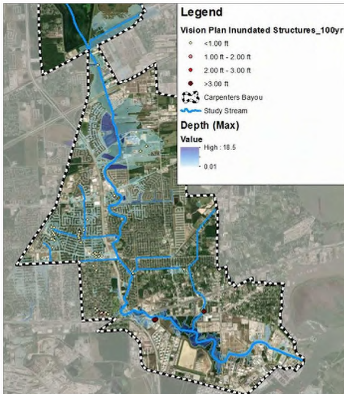
Figure 9. Residual Flooded Structures considered for buyouts under proposed conditions (100-year)
