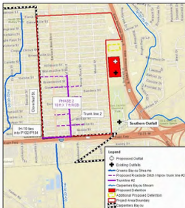
Figure 6. Tie-in Options for trunk line #2
