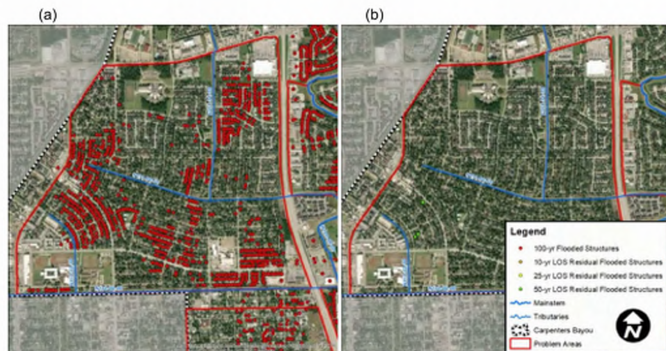
Figure 15: Target LOS alternative Analysis for PA02 (a) 100-year computed flooded structures (b) Computed residual flooded structures after 50-year LOS for PA02
