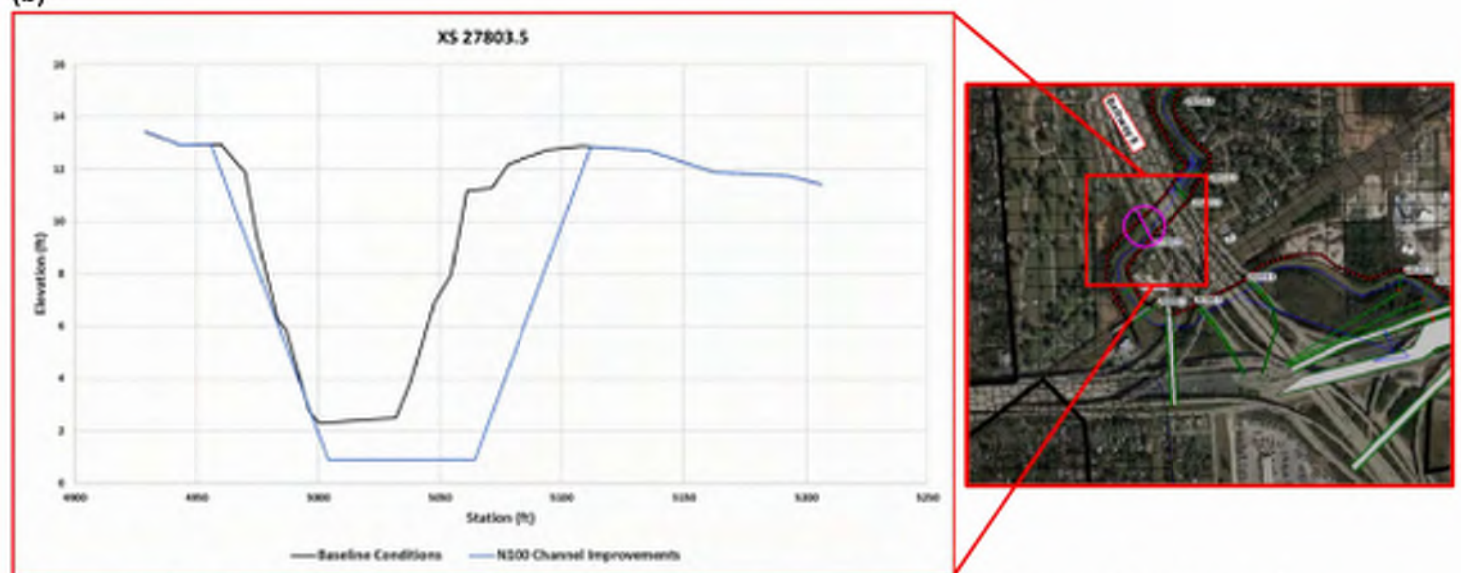
Figure 4. Examples of channel widening across two cross-sections between Baseline and Proposed Conditions (a) Cross-section 30682.5 (b) Cross-Section 27803.5
