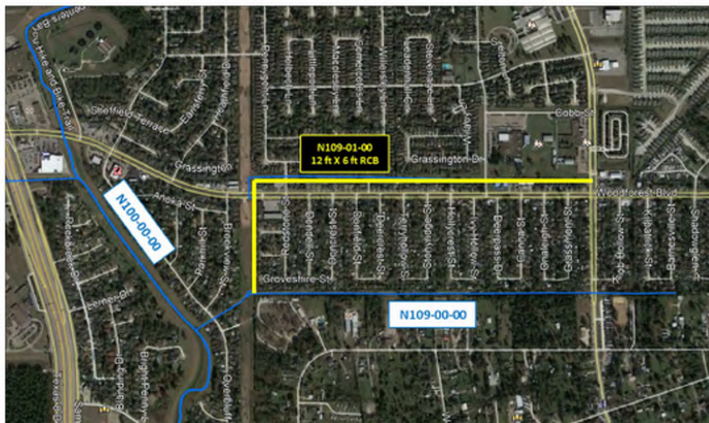
Figure 7. N109-01-00 tributary improvements
