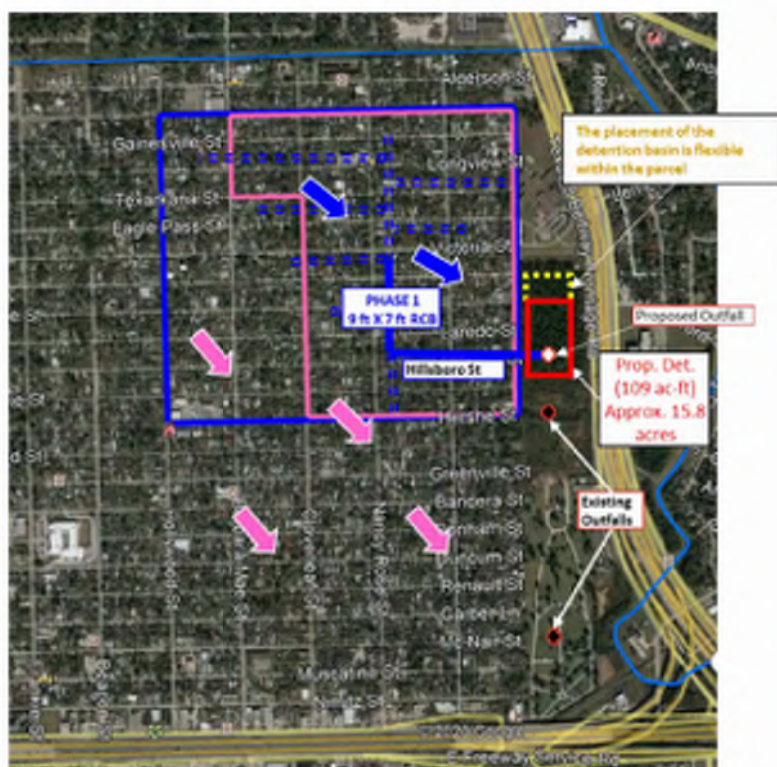
Figure 2. Existing and Proposed Conditions drainage boundaries Phase 1
