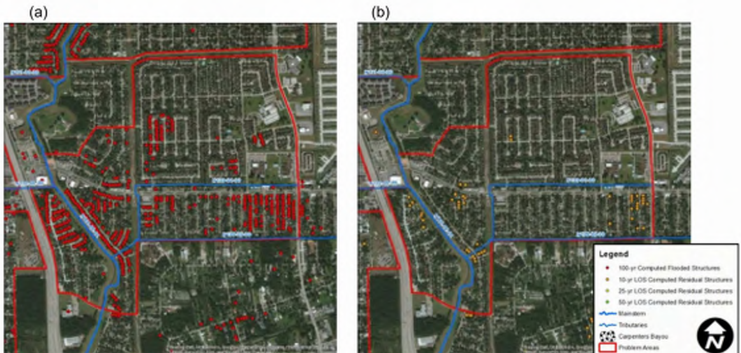
Figure 6: Reduced LOS alternative Analysis for PA01 (a) 100-year computed flooded structures (b) Computed residual flooded structures after 10-year LOS for PA01
