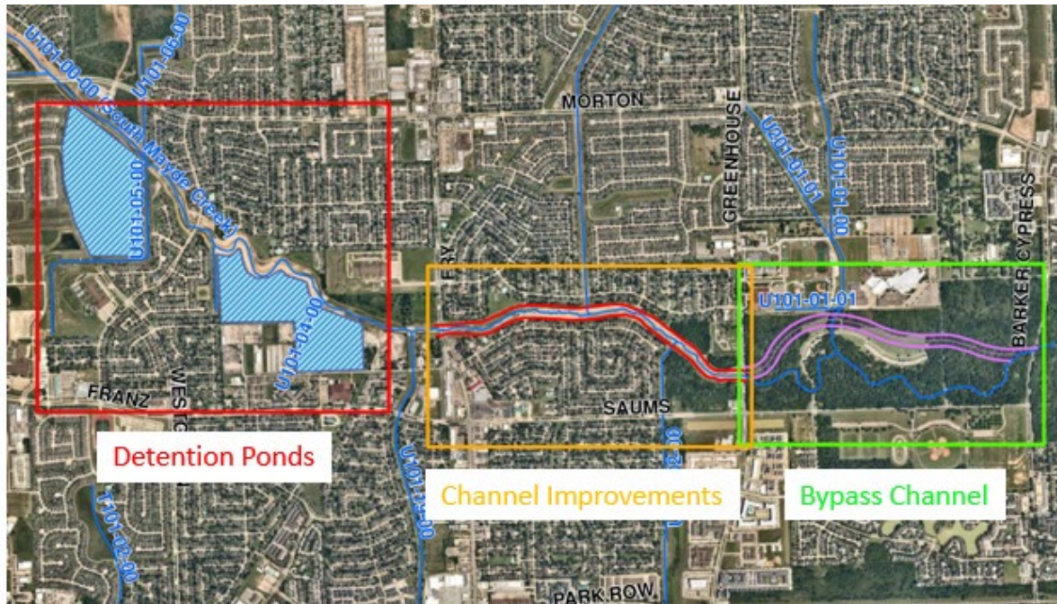
FIGURE 5-32: LOWER SOUTH MAYDE CREEK PROJECT COMPONENTS
