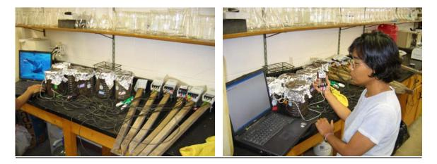
WaterMark sensor calibration in the laboratory to specific soil types (left) was performed to better assess what the optimum sensor reading range is appropriate to know when to irrigate. Irama Wesselman, Environmental Engineering M.S. graduate student (right) worked on sensor calibration and is developing a "fuzzy logic" model that takes into account ET and soil moisture sensor reading to determine when to irrigate fields.
