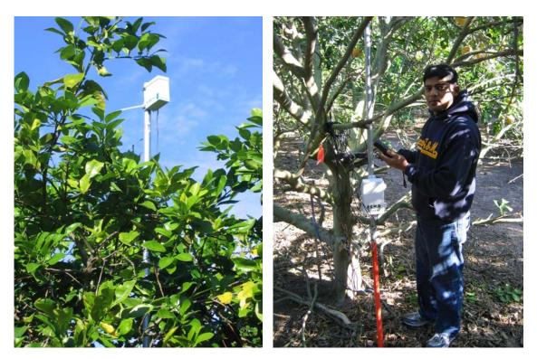
ADI collaborator Juan Ramirez has a citrus farm with mature citrus (Rio Red grapefruit, Blood navel oranges, and tangerine) under flood irrigation. Ram Uckoo, TAMUK M.S. graduate student equipped this EM-50 datalogger with 4 ECH<sub>2</sub>O soil moisture probes (left) and a raingauge attached to the top of a metal pipe extending above the mature citrus tree canopy (left).
