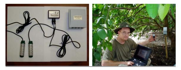
WatchDog<sup>®</sup> dataloggers equipped with WaterMark<sup>®</sup> soil moisture sensors (left) are used at various field locations to track water content within the soil profile over the growing season. Data is downloaded periodically to a computer (right) and some growers have adopted this technology as a means of irrigation scheduling.
